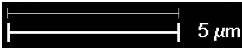
Figure 4.4: Direct comparison between the SEM software scale bar (top) and the application-generated scale bar (bottom), both labelled 5 \mu\text{m} (although not visible in this example). Both bars have essentially the same physical length when measured from end to end in pixels; any residual difference is on the order of a fraction of a pixel and visually negligible.
