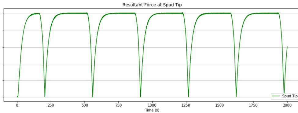
Figure 50 Resultant spud forces for I-dominated controller
