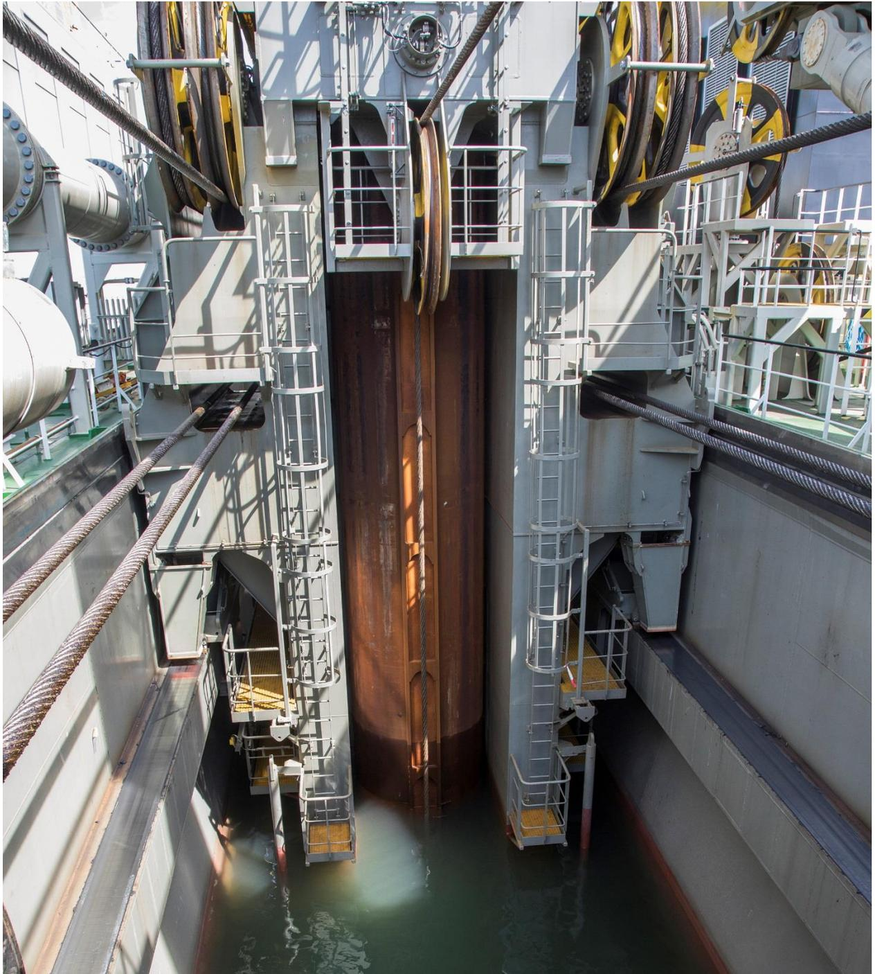
Figure 26 Detailed view of the spud carriage
