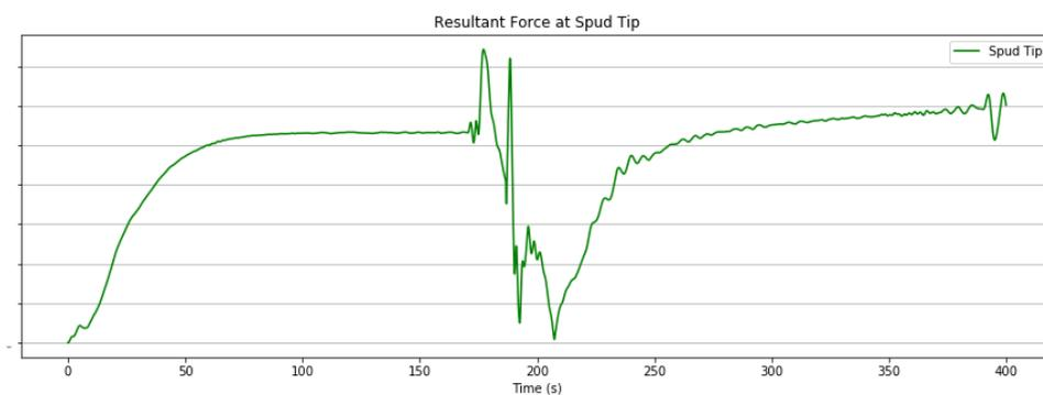
Figure 66 Spud force at full operation
