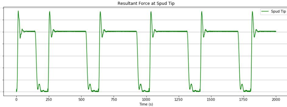
Figure 49 Resultant spud force for P-dominated controller
