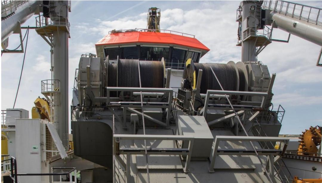
**Figure 38 Winches on top of the ladder provide tension in the side wires**
