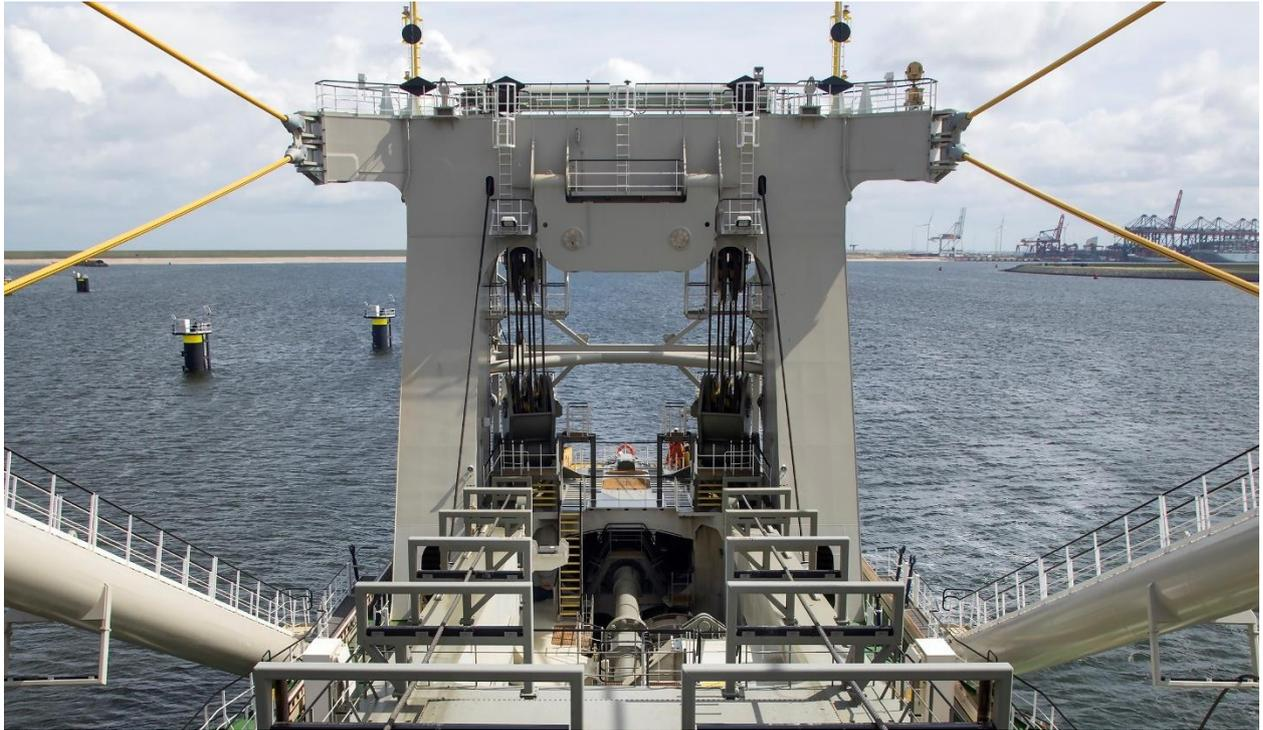
Figure 9 A-frame with hoisting wires visible and ladder hoisted
