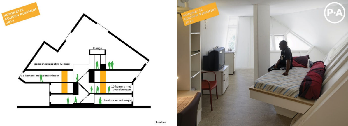
FIGURE 7.11 - SECTION AND PATIENT ROOM OF THE SUPERKUBUS (2014, PERSONAL ARCHITECTURE). IMAGES: WWW.PERSONAL-ARCHITECTURE.NL, ACCESSED 18-5-2015.
