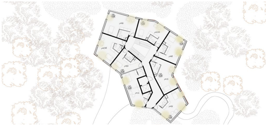
Figure 31. Huis aan 't laar : the irregularity of the plan and placement of the windows allow for natural cross ventilation and distinct views.
