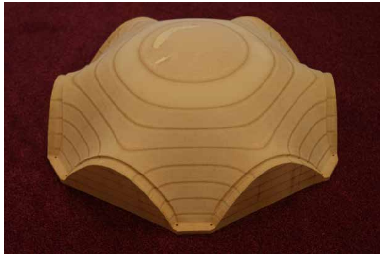
(a) Formwork of Model A (shell with straight supports).
