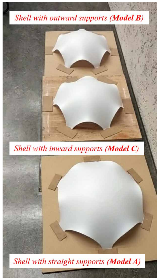
FIGURE 9.6 Three plastic shell models with supports.
