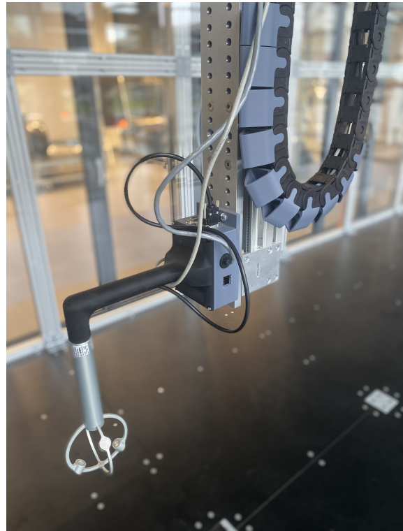
(b) Close-up of a LI-560 TriSonica mounted on the rake for real-time velocity measurements in the Wind Box.
