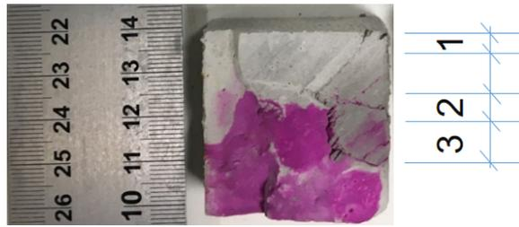
Figure 8.5: The positions where powders were extracted, using slag A18 paste as an example. 1: fully carbonated area; 2: transitional area; 3: mildly carbonated area.
