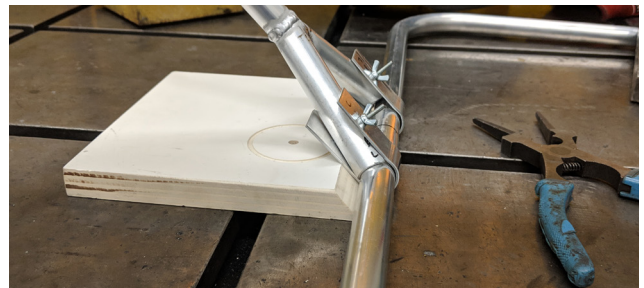
Figure 116 - Bent plates that hold the handlebar put into position before fixing them with aluminum welding
