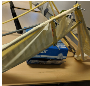
b) Textile showing stress during folding (left), and ripping (right)
