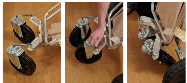
Figure 118 - Cut and bent sheet metal with wood in between serving as attachment points for the pivoting wheel Attachments
