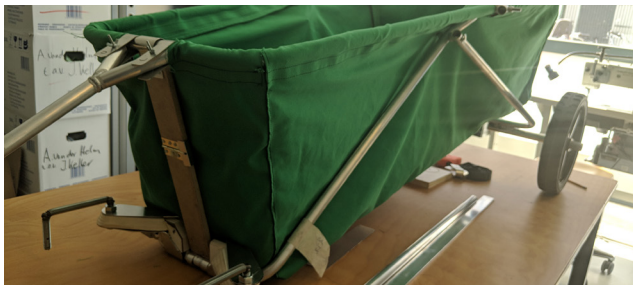
Figure 119 - The pivoting front boards with a 'lock' keeping the hinge in place to simulate the locking and unlocking of the front gate.
