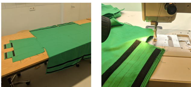
Figure 120 - The cut textile being sewn with black velcro attached
