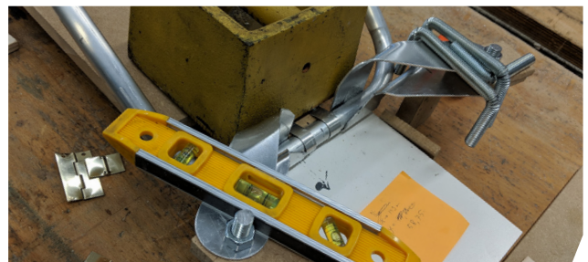
Figure 117 - Cut and bent sheet metal being metal glued to the frame
