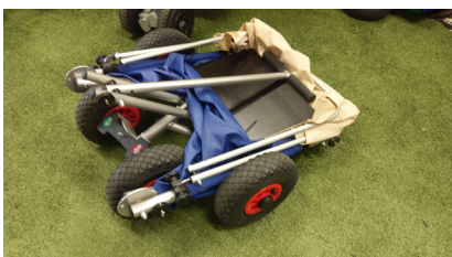
Figure 8 - Folded hand cart unable to stand
