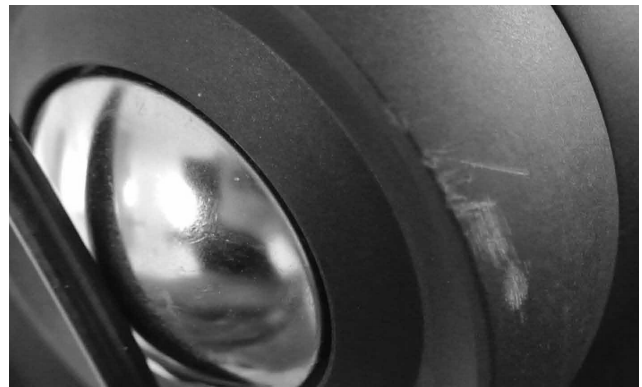
Figure 54 - A refurbishable part showing scratches as aesthetic wear (Keijzers, 2013)
