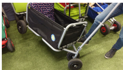
Figure 12 - Little force makes cart tip over
