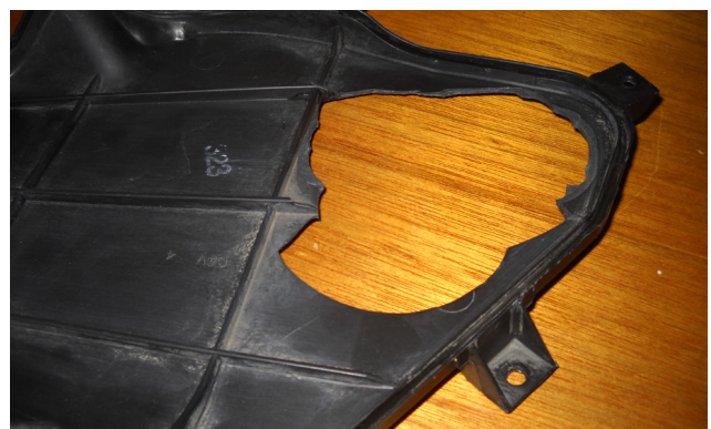
Figure 55 - A part unsuitable for refurbishment, showing functional breakage (ProvideYourOwn, n.d.)
