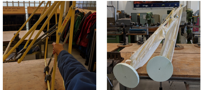
Figure 92 - Bottom moves out of vertical plane due to unequal diagonal bottom lengths (left). Wheels folding at unequal height due to unequal diagonal beam lengths (right).
