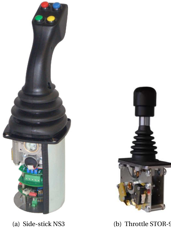
Figure 3.1: Side-stick and throttle manufactured by Spohn & Burkhardt GmbH & Co.
