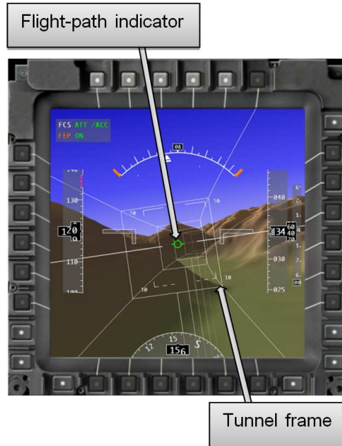
Figure 7.15: SAFAR primary flight display, developed by dr. ir. C. Borst
