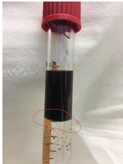
Figure 10: Crude oil and demineralized water test. The circled area shows a small micro-emulsion layer observed after 24 hours
