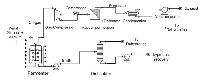
Ethanol recovery from fermentation off-gas by vapour permeation with recovered ethanol fed to distillation.
