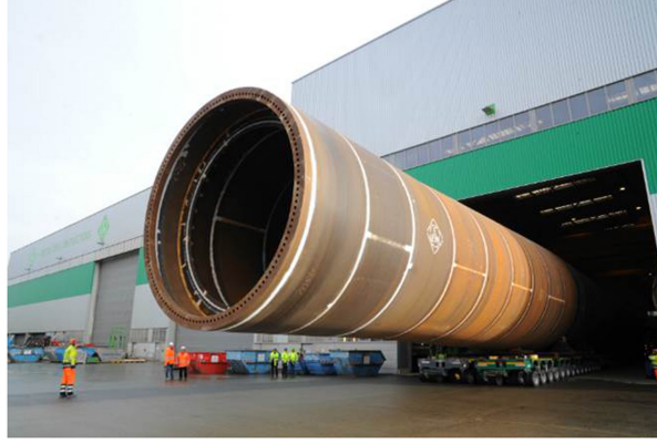
Figure 1.2: Monopile foundation for an offshore wind turbine [5]
