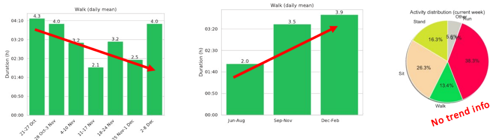
Figure 3.7: Example plots to illustrate the trend feature ( q_{tre} ): the first figure has an overall negative slope (i.e trend), second has a positive trend, and no trend value can be determined for the third type of plot.
