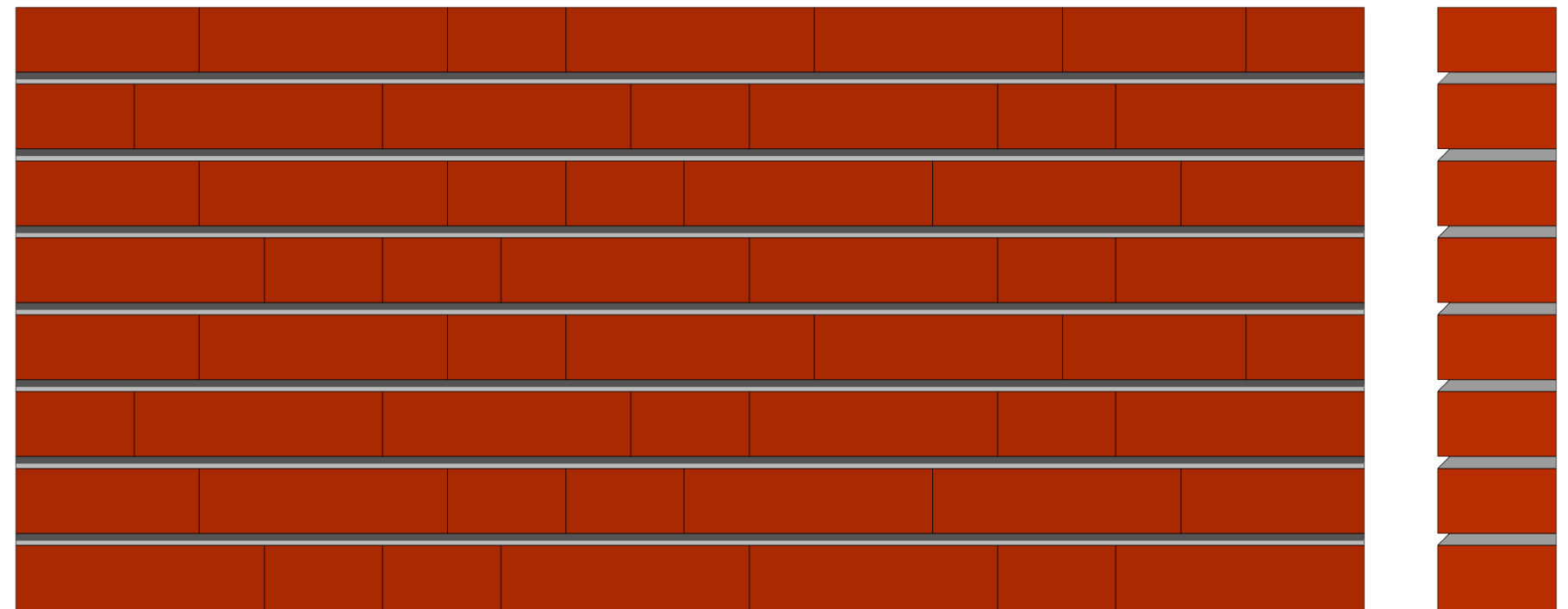
Horizontal brickwork, in wild bond, with a weather joint; study image
