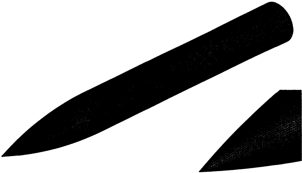
Figure 6.32: Surface grid of the ogive cylinder (17,893 nodes), entire and zoom near the apex.
