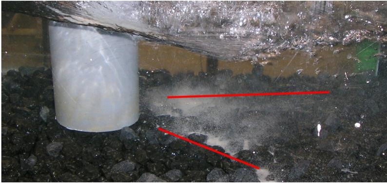
**Figure 5-19 Erosion behind a round pile (red lines indicate the diverging turbulent motion)**
