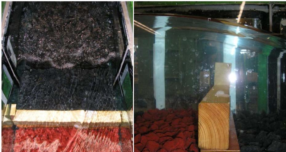
**Figure 4-13 Sill (left: top view (flow direction: from bottom to top), right: side view (flow direction: from left to right)), height sill: 6,5 cm**
