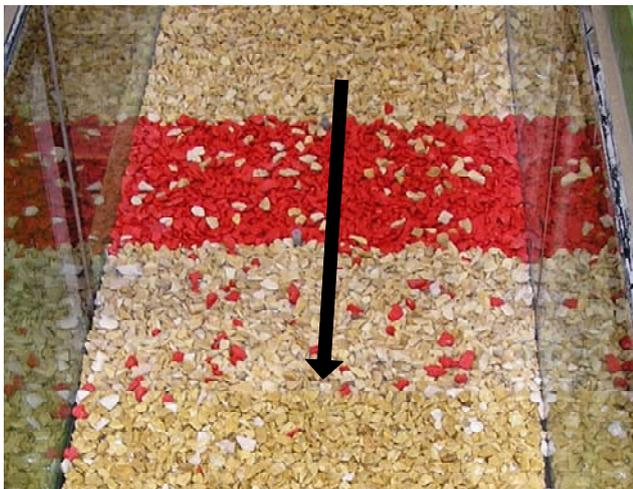
**Figure 4-4 Transport of filter material (black arrow indicates main flow direction)**
