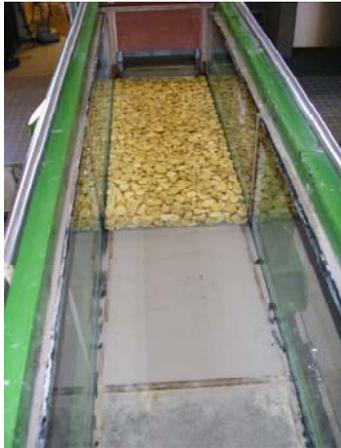
**Figure 4-11 Sand bed between two concrete slabs with on top slabs of stones (glued together with elastocast)**
