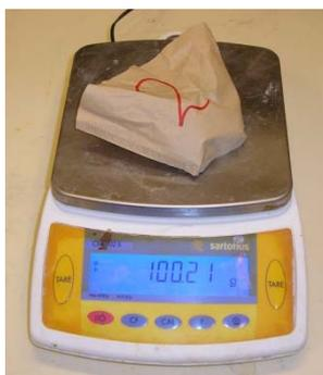
**Figure 4-8 Weighing the sand collected in a sieve**
