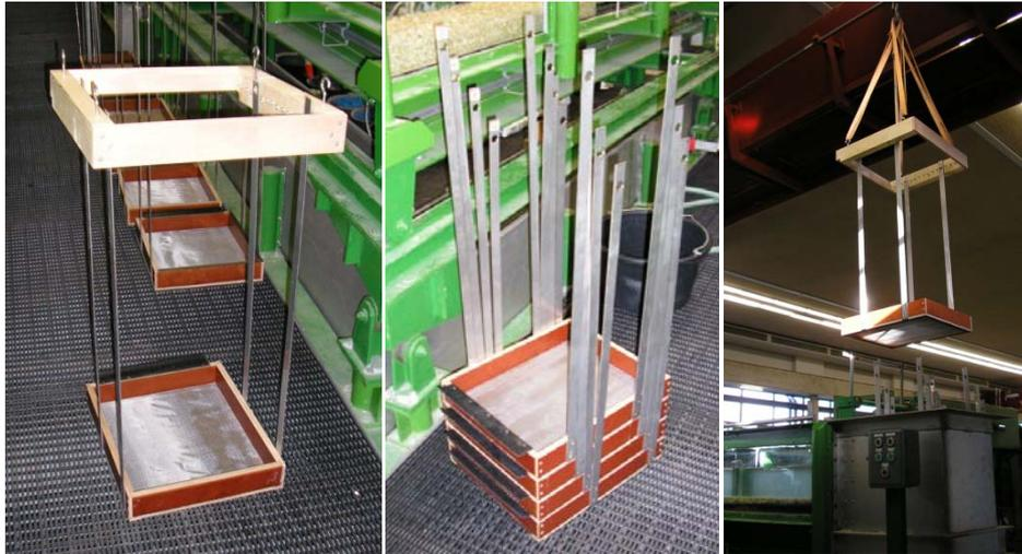
**Figure 4-7 Left: Sieve with lifting frame, Middle: Stack of sieves, Right: Sieve placed with a crane**
