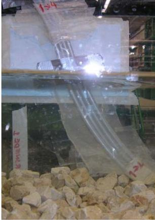
**Figure 5-21 Pressure tubes attached to the flume wall**
