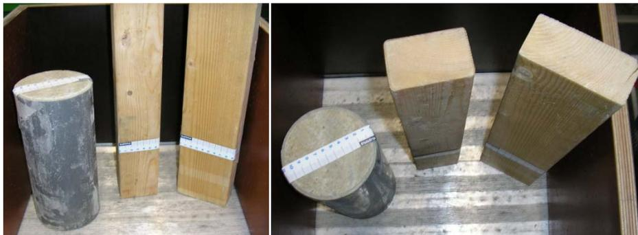
**Figure 4-14 Round and rectangular piles used to increase the turbulent intensity**
