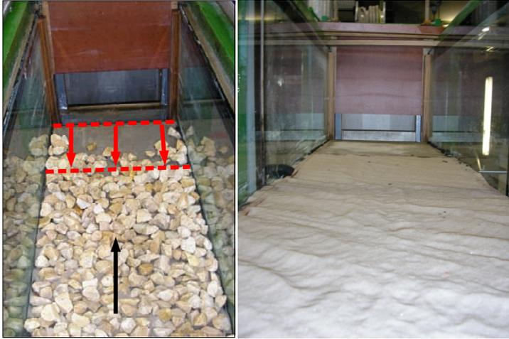
Figure F-3 Left: Retreating filter layer test T02b (black arrow indicates main flow direction), Right: Base layer after the test (after removing the filter layer, test T02a)
