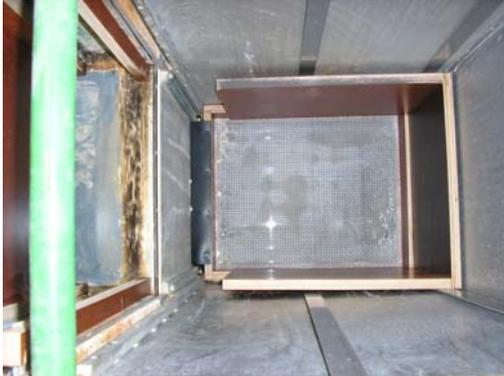
**Figure 4-5 Sieve in the drain of the flume**
