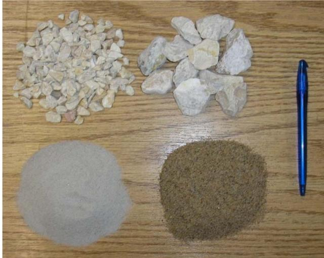
**Figure 4-15 Materials, top: filter material (left: Yellow Sun 8-11, right: Yellow Sun 20-40), bottom: base material (left: m32, right: 0.50-0.80)**
