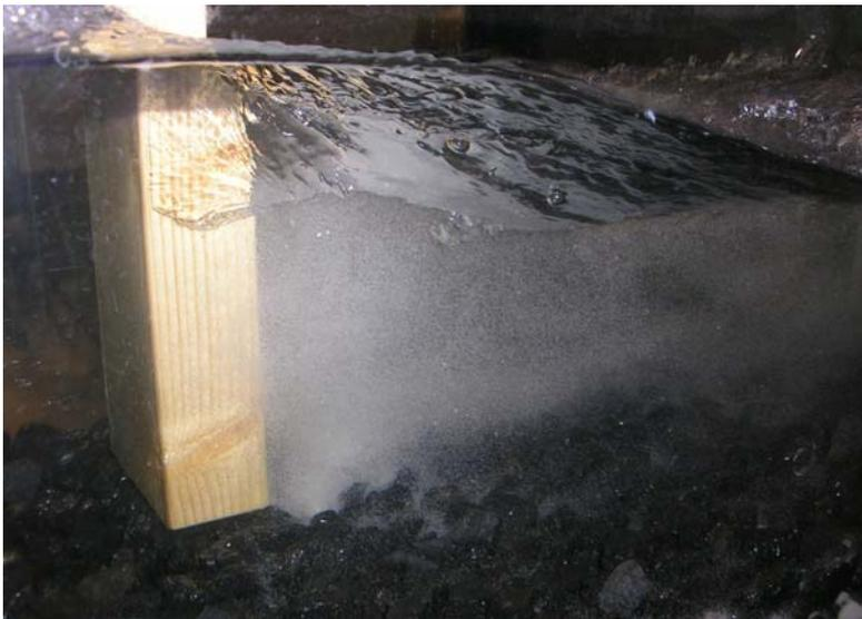
**Figure 5-20 Erosion behind a rectangular pile**
