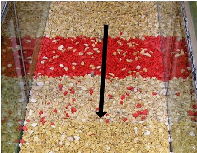
**Figure 5-7 Transport of filter material, test T01 (black arrow indicates main flow direction)**
