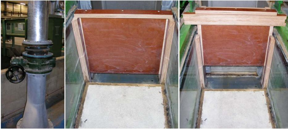
**Figure 5-22** Left: Valve (discharge), Middle and right: Weir (manually)
