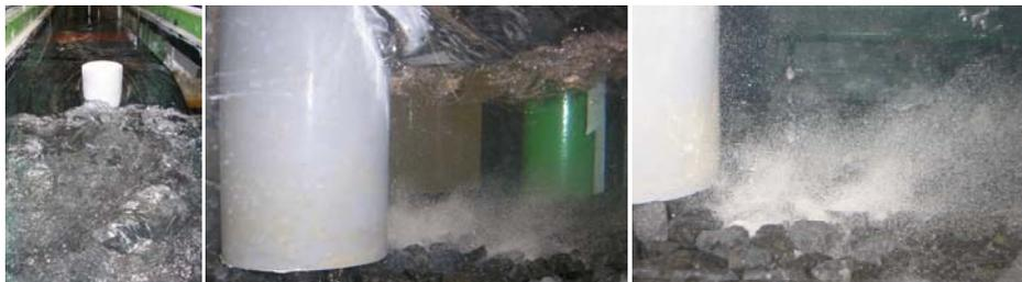
**Figure 5-18 Turbulent motion and erosion behind a round pile**
