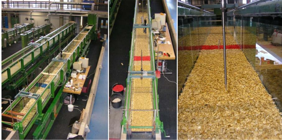
**Figure 4-3 Flume with test set-up in the Environmental Fluid Mechanic Laboratory**
