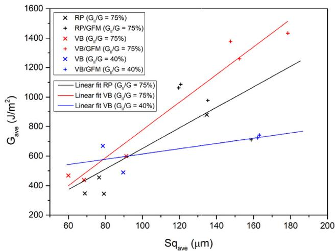
Fig. 16. Relationship between surface roughness and fracture energy.
