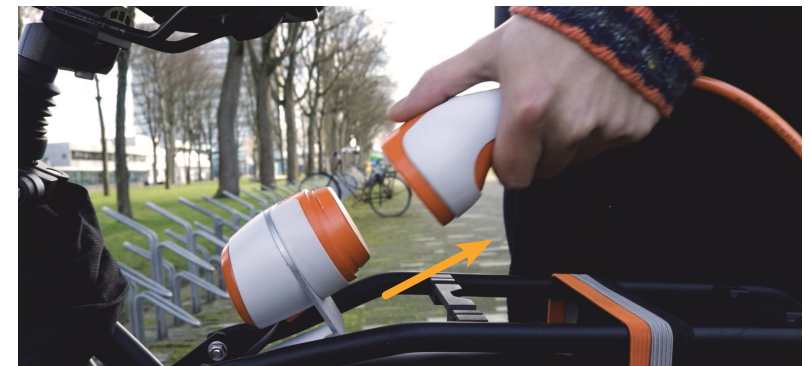
figure 9.7 The click mechanism locks the transmitter in place when pushed downward, but unlocks easily when slightly lifting the handle while disconnecting
