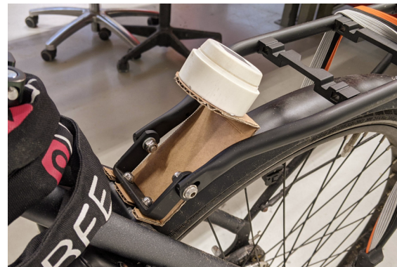
figure 13.7 Cardboard prototypes for the bike bracket were made to ensure correct placement and dimensions
