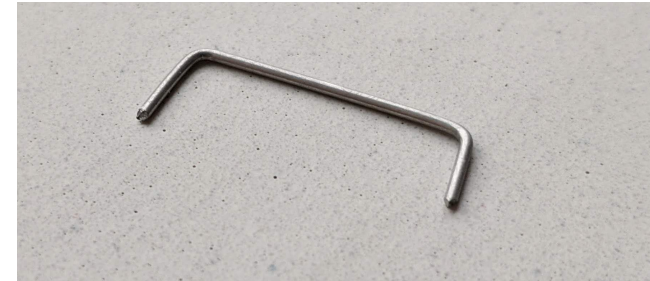
figure G.10 Minimal form of the spring wire to work properly
