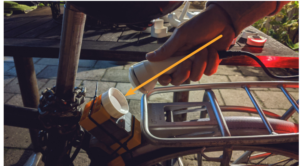
figure 9.3 A linear connection mechanism simplifies the connection and disconnection processes
