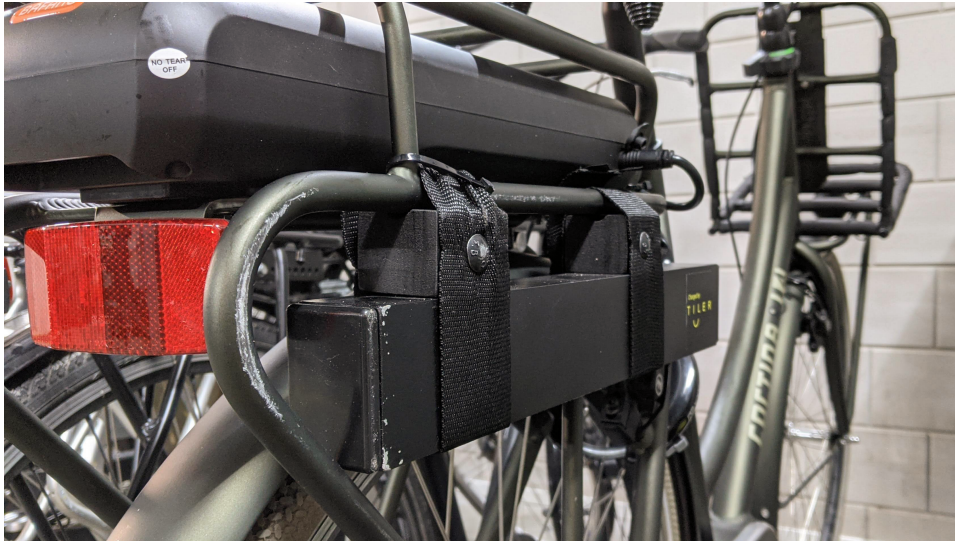
figure 11.5 The bike electronics are currently still relatively large and require an extra container to place them on the bike
