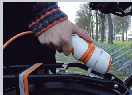
Step 5 The user disconnects the charger and places the transmitter handle back in its docking station that is installed in the hub, right next to the bike
