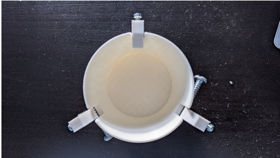
figure G.6 Mechanism with three click fingers does not provide the correct feedback
