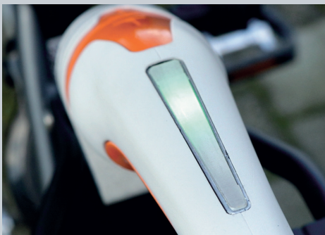
Step 4 Once a bike is reserved, an animated 'stream' of green light is shown to indicate it needs to be disconnected
