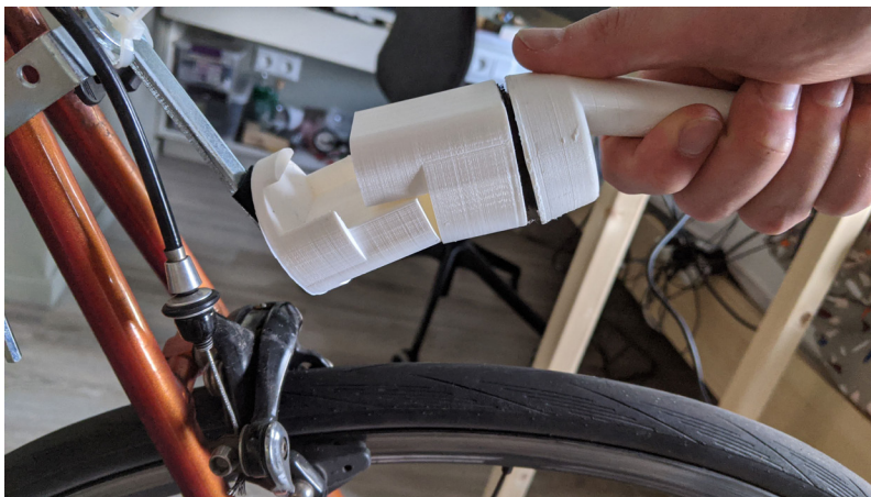
figure F.6 Connection mechanism H was disliked for its precise alignment
