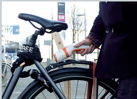
Step 2 The user connects the charger manually by clicking the transmitter handle (handheld) on the receiver (installed on the bicycle)
