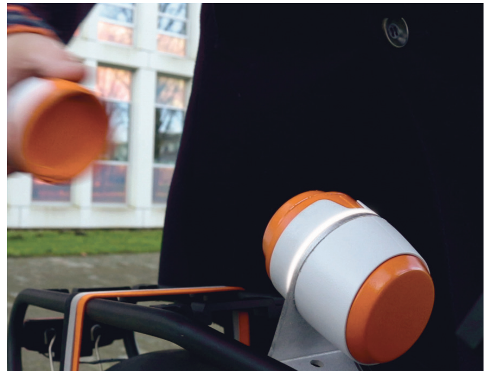
figure 10.6 A light ring is integrated in the receiver to attract attention when the user needs to connect the charger or when a bike is stolen
