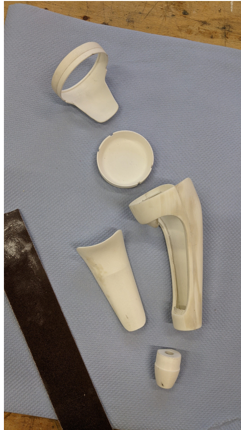
figure H.4 The 3D printed body after sanding and surface finishing
