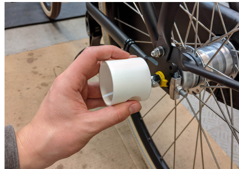
P Wheel axle mount + Easy access - Low and vulnerable - Cables
