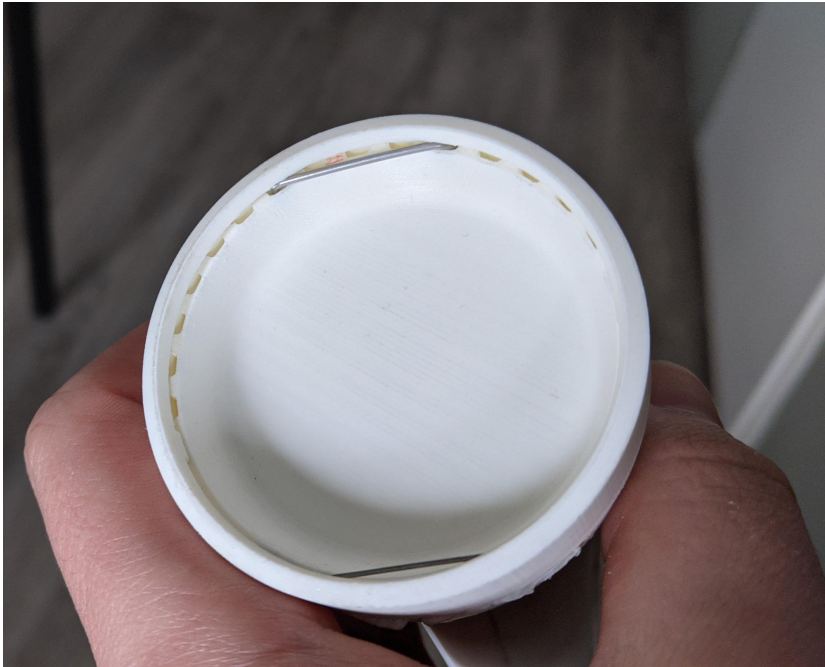
figure G.9 Two spring wires of different thickness ensure correct feedback will always be given to the user
