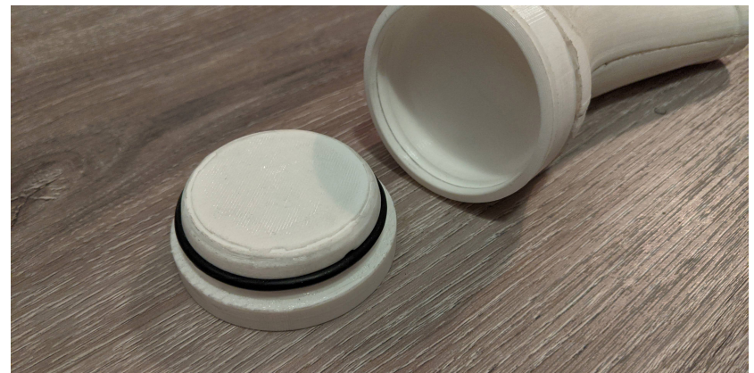
figure G.2 Prototype with a rubber ring on the receiver and a groove on the transmitter side
