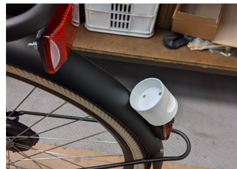
U Rear fender - rear - angled + Easy access + Combination with rear light - Vulnerability
