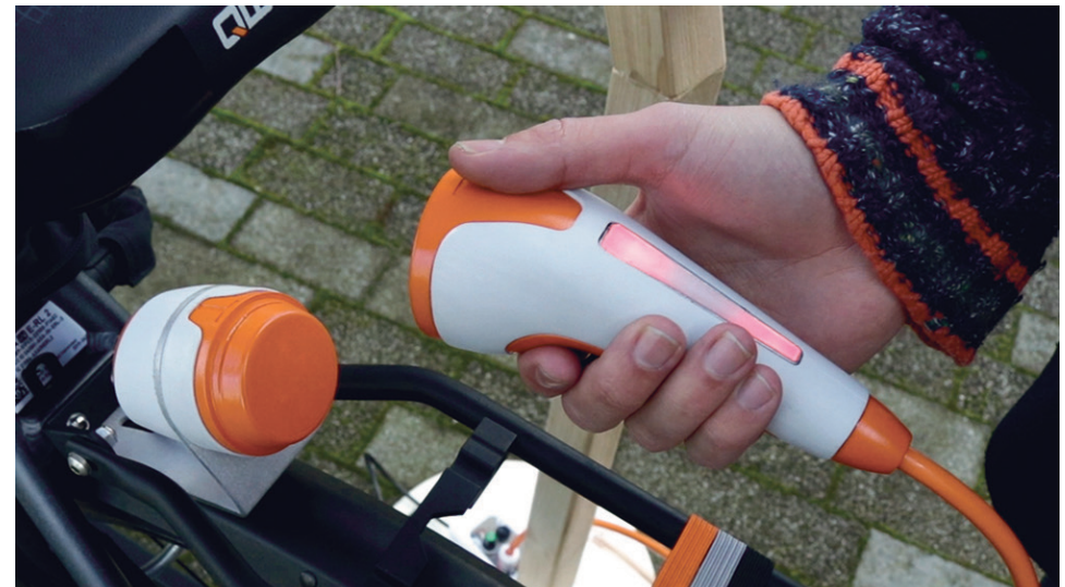
figure 10.8 The light on the transmitter starts flashing red to notify something is wrong and the charger needs to be reconnected to the bike
