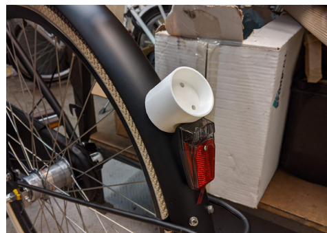
T Rear fender - middle + Easy access + Combination with rear light - Vulnerability
