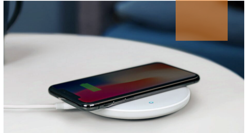
figure 7.6 Wireless charging is usually based on having a portable receiving device that is moved to align to a stationary transmitter
