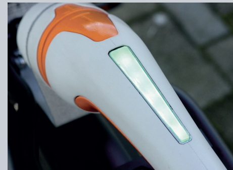
Step 4 If verification of the vehicle is confirmed, the light element flashes green a couple of times to indicate that the lock may now be closed
