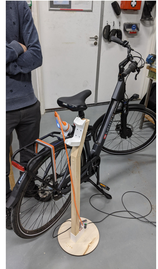
figure H.6 Semi-improvised charger pole
