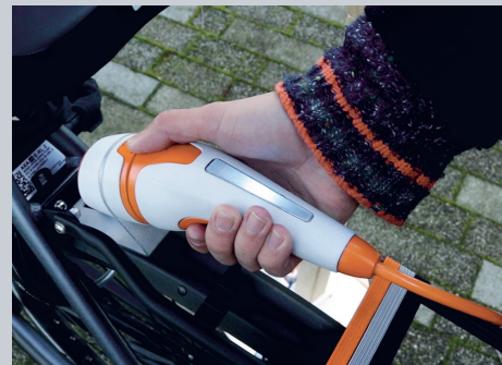
Step 3 The charger recognizes that it is connected and verifies the vehicle's ID to make sure the vehicle is allowed to charge in the specific hub
