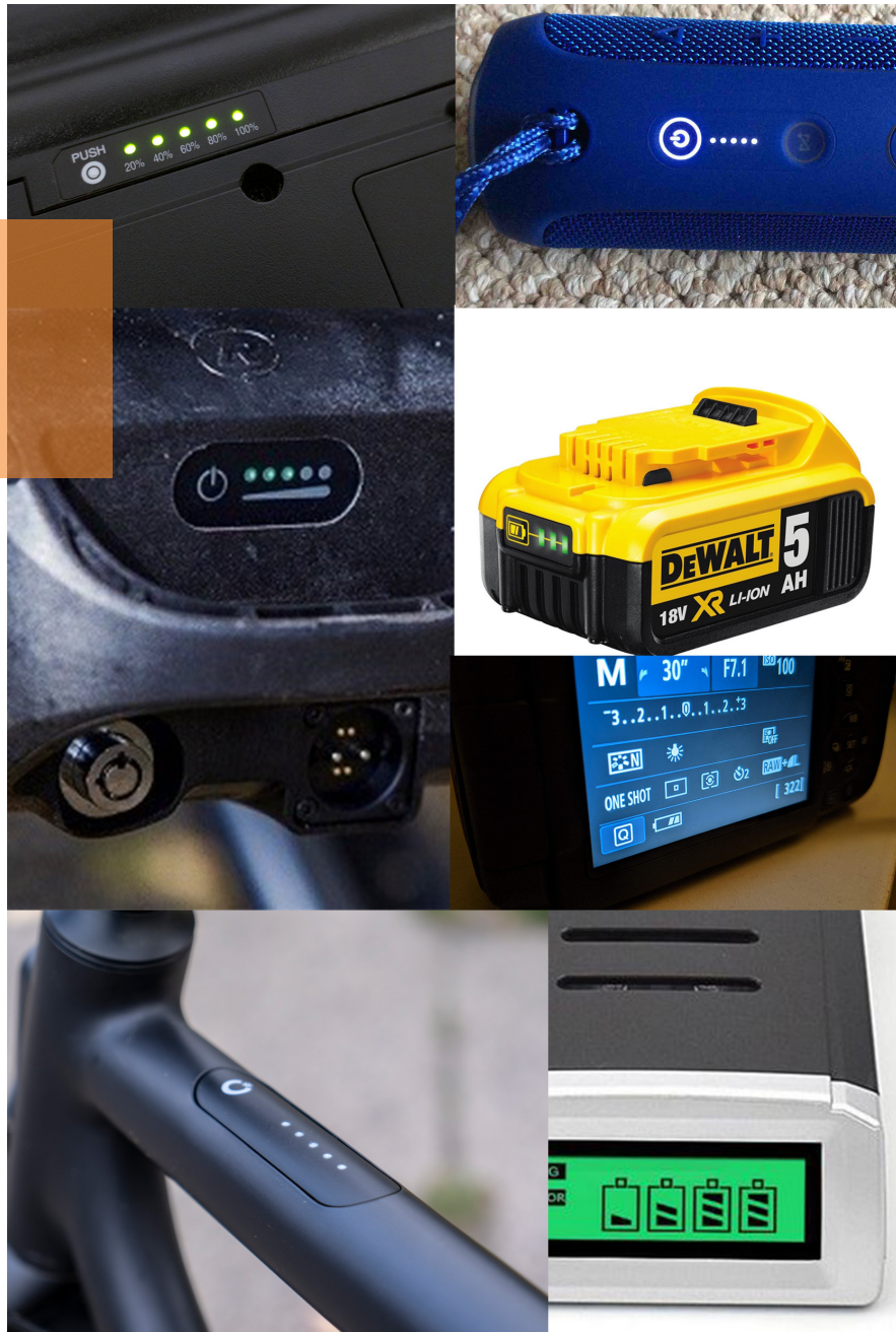
figure 10.3 Using multiple LEDs to communicate battery level is fairly common in all sorts of applications
