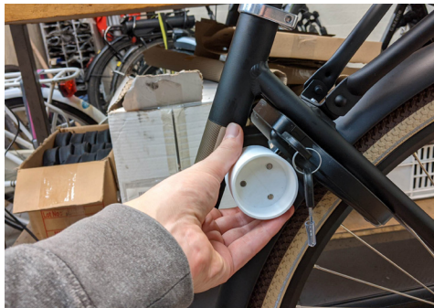
O On frame - seat post + Easy access - Not a lot of space for some bikes
