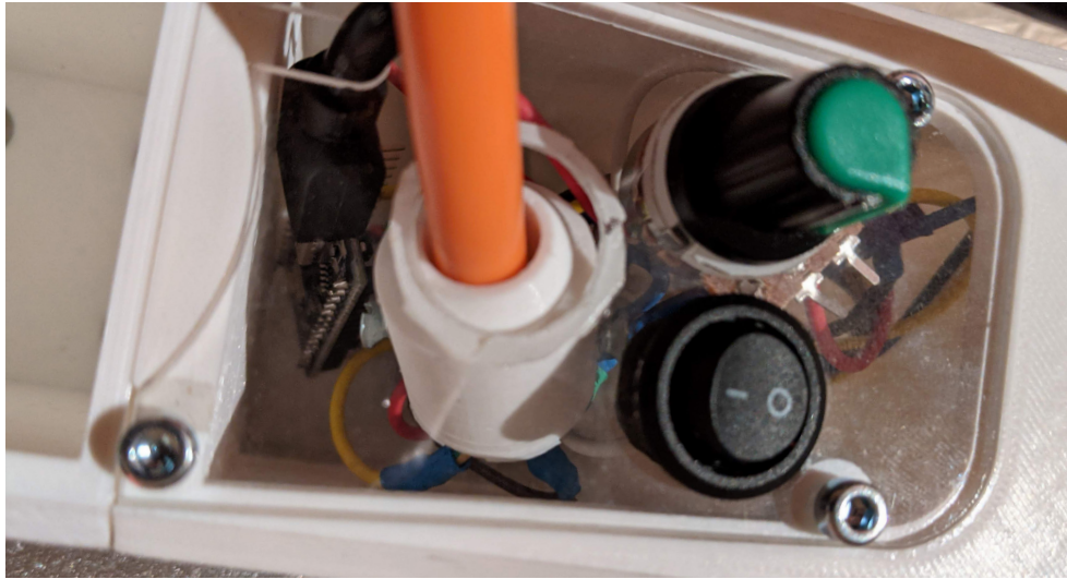
figure H.7 The charger pole houses a second Arduino and a switch button to simulate reservation status
