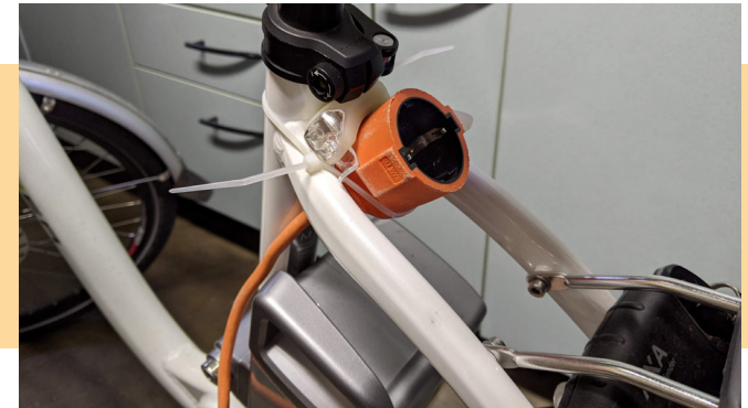
The end of an extension cable has been placed on the anticipated place of the receiver in the concept.
