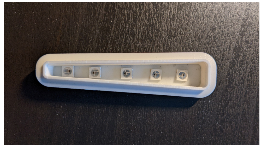
figure H.2 Five Neopixel RGB LEDs are placed in line in the light display
