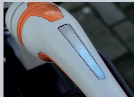
Step 6 The light element indicates the current battery level, while the last LED is flashing to indicate it is charging
