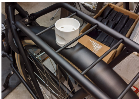
S Rear fender - middle + Easy access - Vulnerability - Combination with rear carrier (could be +)
