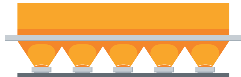
figure 10.2 Multiple LEDs light the light surface from a slight distance to generate a visually uniformly lit surface
