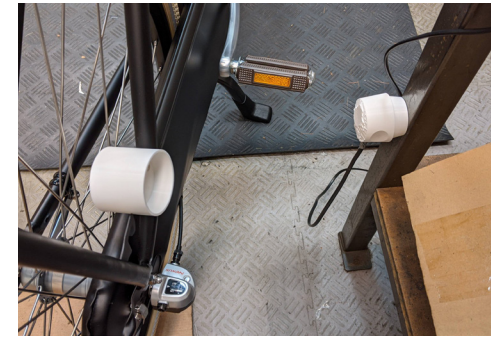
N On frame - On top of rear fork - Vulnerability (extreme) - No space for wheel covers
