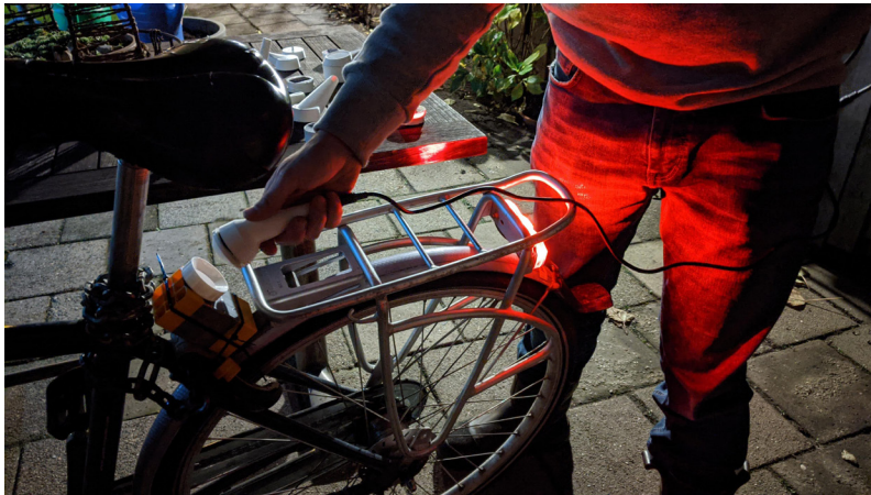
figure F.5 Handle design 8 with a linear connection mechanism that prolongs the movement of transmitter towards receiver in the connection
