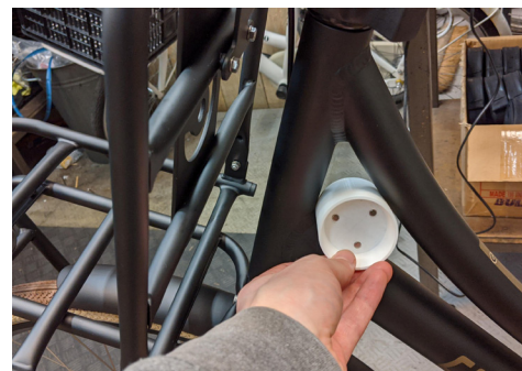
H On frame - front - angled - Hard to reach from back of bike - Not universal
