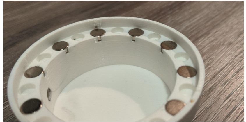
figure G.1 Tests setup with multiple small magnets inside the embodiment that surround the ferrite core
