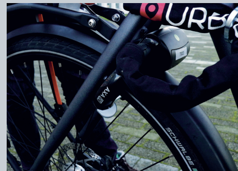
Step 6 Once the charger is disconnected, the smart lock opens automatically, allowing the user to take the bike out of the bike rack
