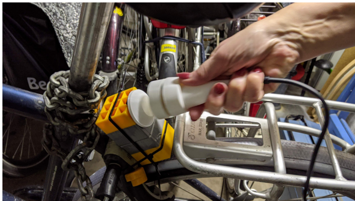
figure F.3 Example of an improvised mounting plate
