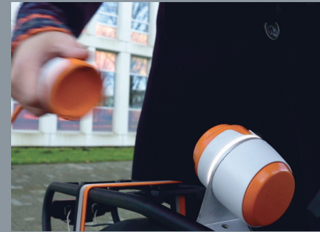
Optional If the mobile application is used to end the ride, the integrated lighting inside the receiver starts flashing to attract the user's attention towards the charger
