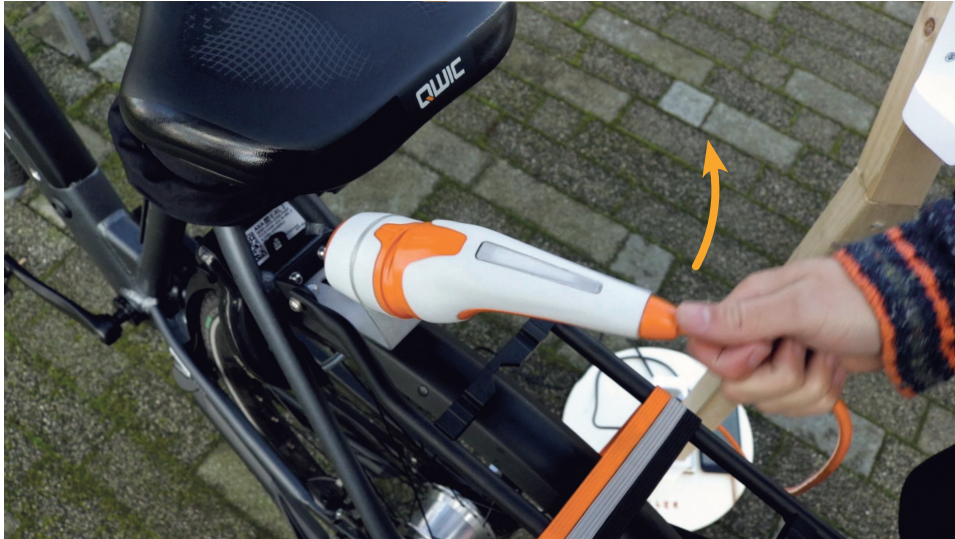
figure 9.8 Though locked in place while charging, the clicking mechanism unlocks when the cable is pushed aside (e.g. when someone trips over the cable)
