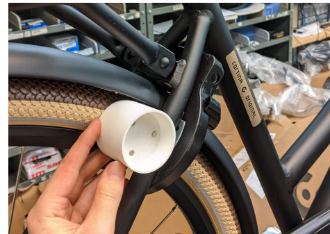
Q Between frame and lock + Use existing mounting option + Users also interact with lock, same place
