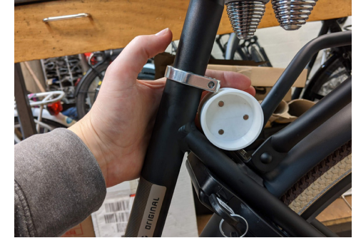
B Integration with seat clip - angled + Universal + Easy access - Usually the place of the chain lock
