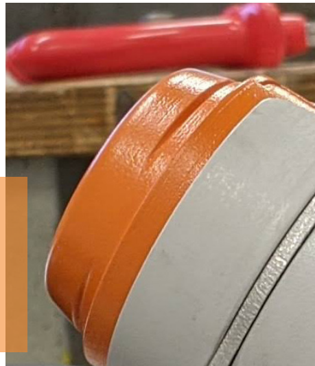
figure 9.6 The geometry of the upper groove differs slightly from that of the lower groove to allow easy disconnection
