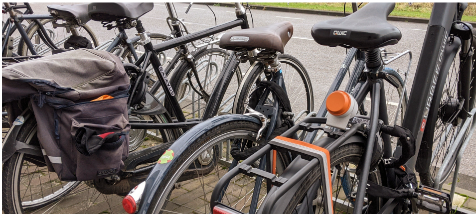
figure 8.1 Receiver placement on the rear provides visibility and easy access from behind the bicycle, e.g. when no space is available between bikes
