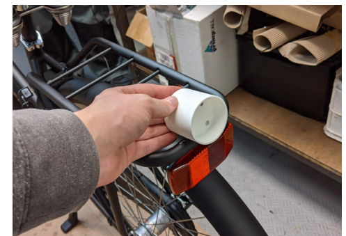
V Rear carrier + Easy access + Replaces reflector/combination rear light - Many bikes have no rear carrier (misuse)
