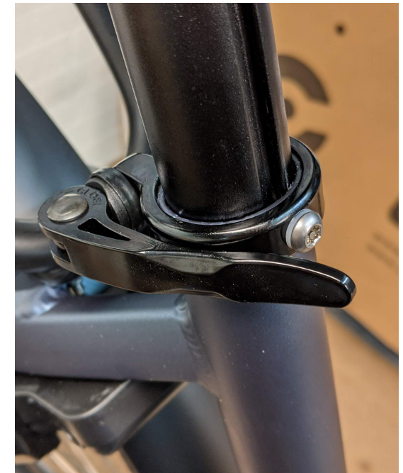
figure D.28 Quick-adjust seatpost-clip that is locked to the bike
