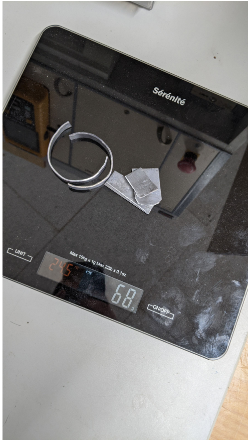
figure H.3 Added lead mimics the weight of the ferrite core
