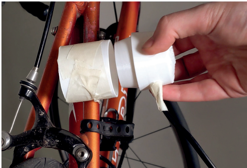
figure 7.1 The initial concept of the Wireless Cable is based on a movable transmitter coil, connected through a cable to a stationary charger pole
