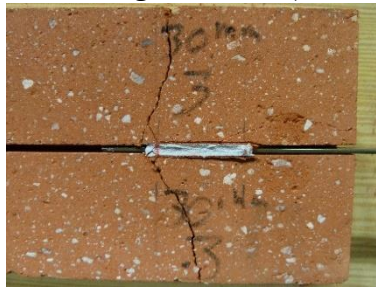
B (Full debonding with diagonal cracks)
