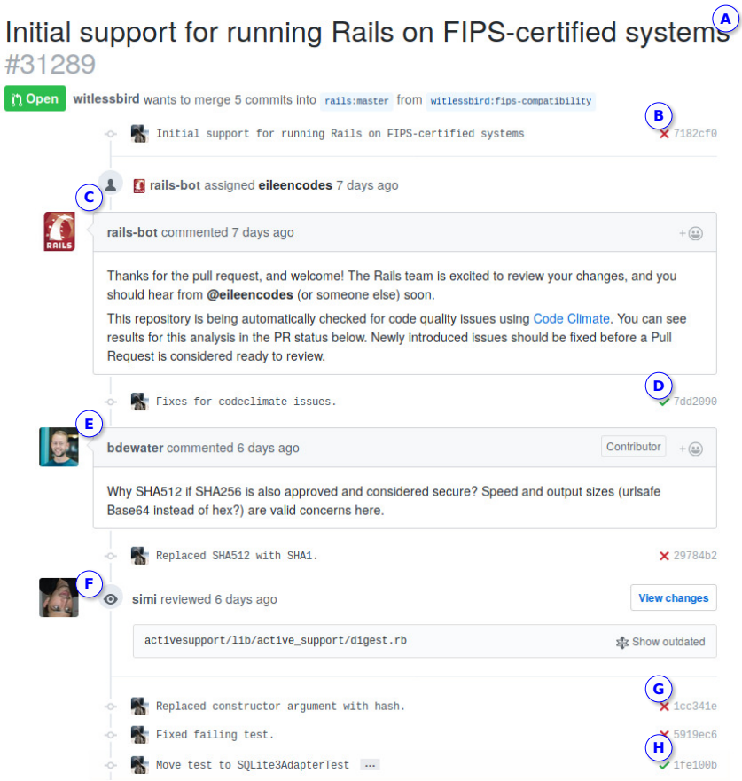
Figure 1.3: A constructed exemplary pull request of the RUBY ON RAILS project showing feedback loops and their integration into pull-based development in action.
