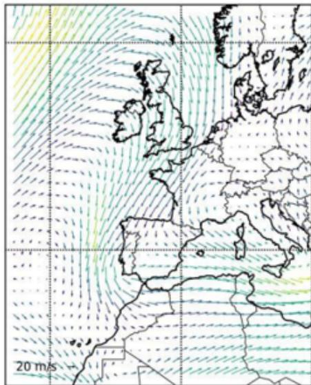
Figure 3.6: Example output of GRIB file data extraction - wind vectors. EUROCONTROL.
