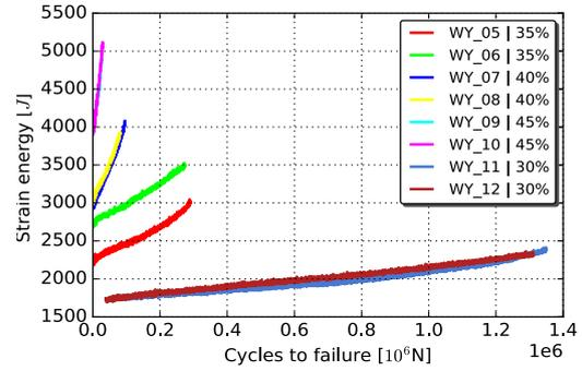
Figure 5: Strain energy vs cycles to failure.
