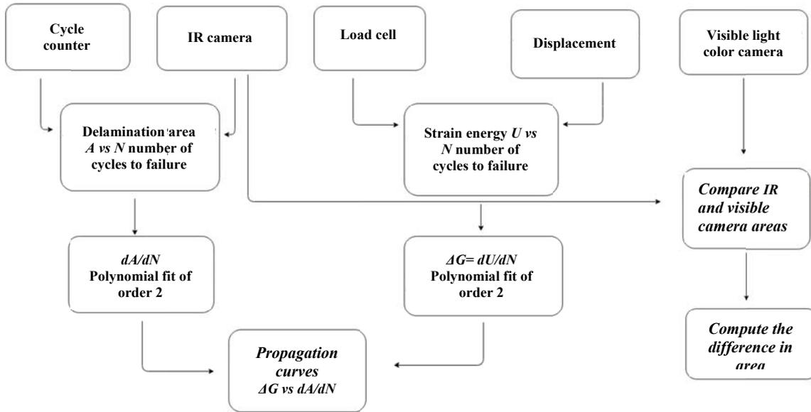
**Figure 3: Test process flow to arrive at fatigue growth curves.**
