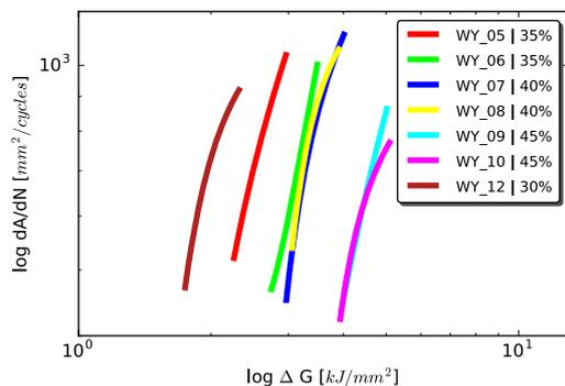
Figure 6: Propagation curves  $(dA/dN$  vs  $\Delta G)$ .
