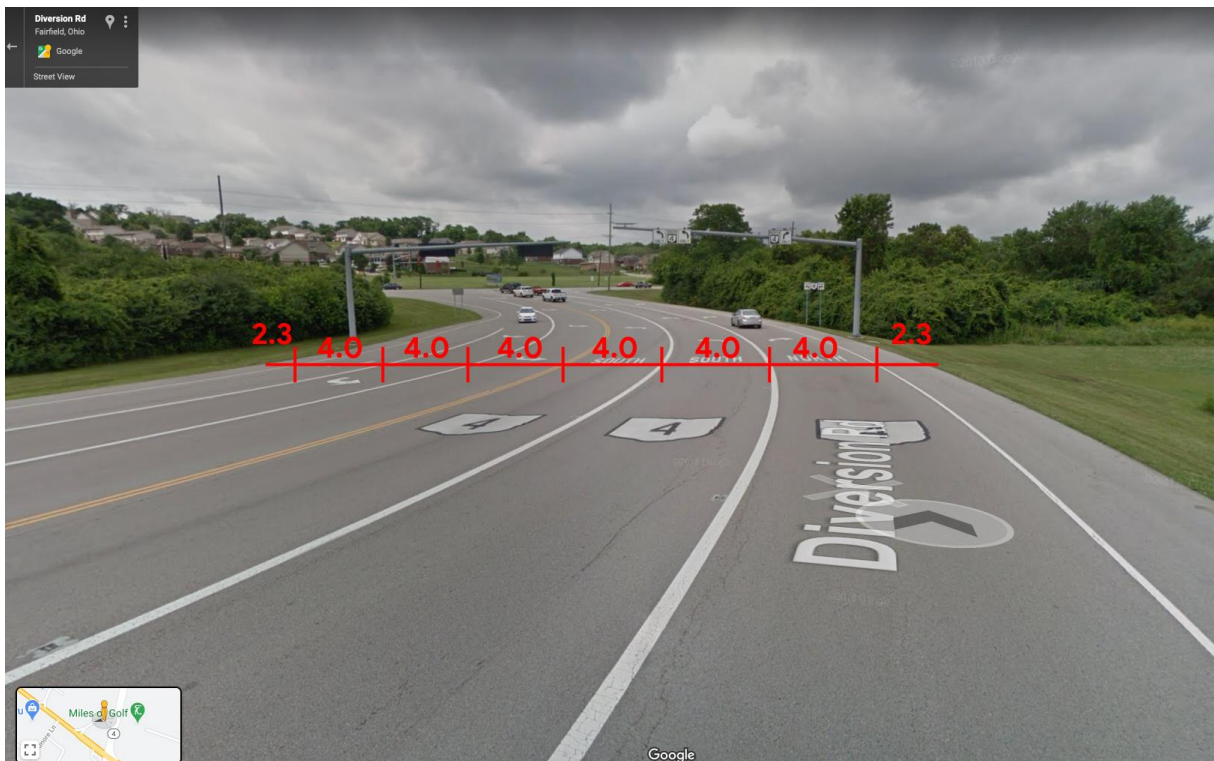
Figure 81 All lane types that do not comply with the Dutch guidelines.
