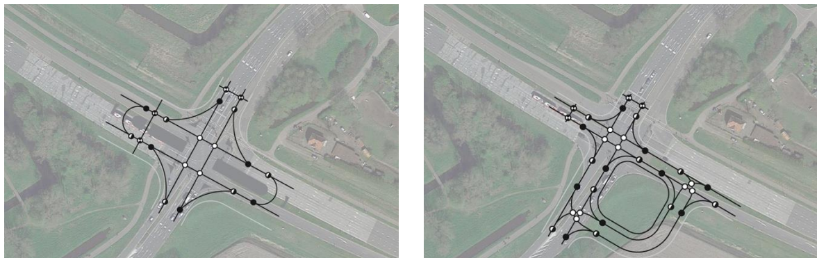
Figure 34 Conflict points plotted on location 1 (not on scale). Left: MUT. Right: QR
