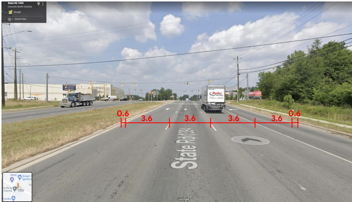
Figure 79 All lane types that do not comply with the Dutch guidelines.
