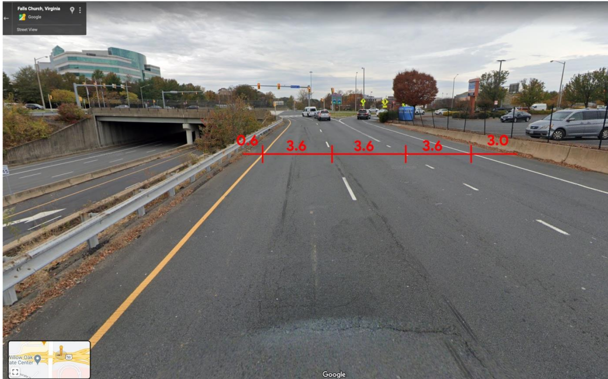
Figure 2 Dimensions of an exit that does not comply with the Dutch guidelines.
