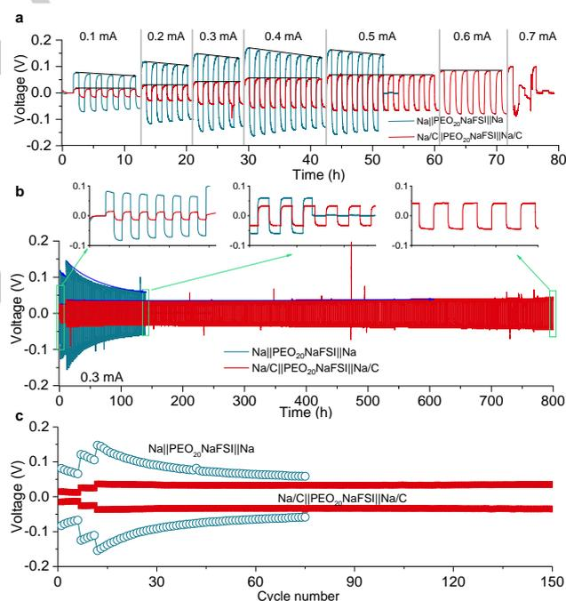
**Figure 2.** Galvanostatic cycling of symmetric  $\text{Na}||\text{PEO}_{20}\text{NaFSI}||\text{Na}$  and  $\text{Na/C}||\text{PEO}_{20}\text{NaFSI}||\text{Na/C}$  cells at  $80^\circ\text{C}$ . (a) Rate performance from 0.1 to 0.7 mA. Comparison of the (b) long-term cycling stability of symmetric cells and (c) voltage curves of the first five cycles at a current density of 0.1 mA, the second five cycles at a current density of 0.2 mA, and subsequent cycles at 0.3 mA.
