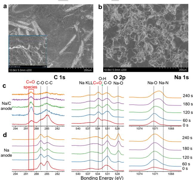
**Figure 5.** Interface properties after 100 cycles in full cells. SEM images of the Na anodes from (a) Na/C||PEO<sub>20</sub>NaFSI||Na<sub>3</sub>V<sub>2</sub>(PO<sub>4</sub>)<sub>3</sub> cell and (b) Na||PEO<sub>20</sub>NaFSI||Na<sub>3</sub>V<sub>2</sub>(PO<sub>4</sub>)<sub>3</sub> cell after 100 cycles. XPS C 1s, O 2p and Na 1s spectra for (c) composite Na/C anode and (d) Na-metal anode from full cells.
