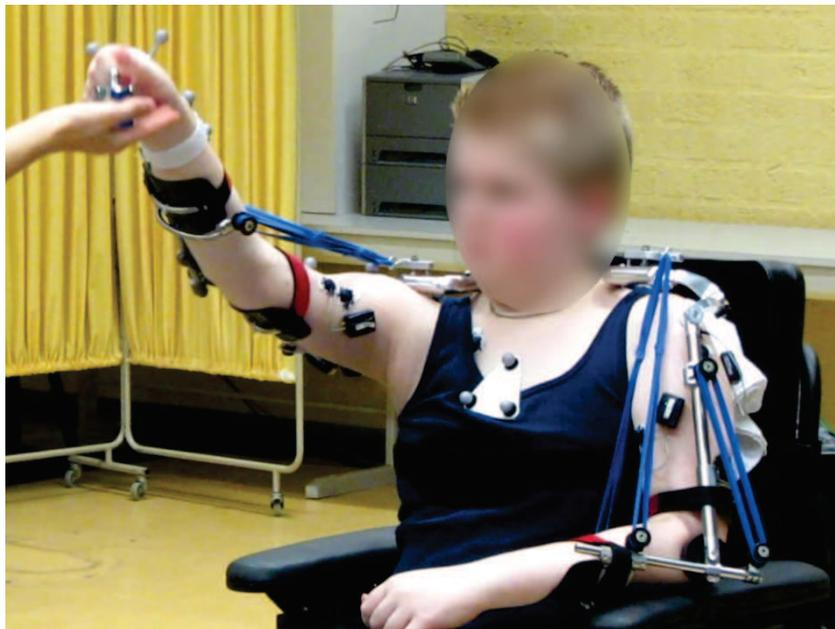
Figure 11.4: Boy with Duchenne testing the prototype, while wearing electromyography and motion capturing devices.
