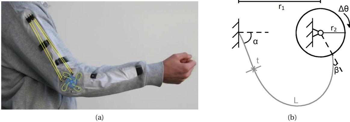
Figure 6.3: The prototype (a), with the antagonistic actuator (yellow) along the upper arm and the compliant rotational joint (green) attached at the elbow of an artificial arm and (b) a schematic representation of one preloaded leaf spring in the compliant rotational joint.
