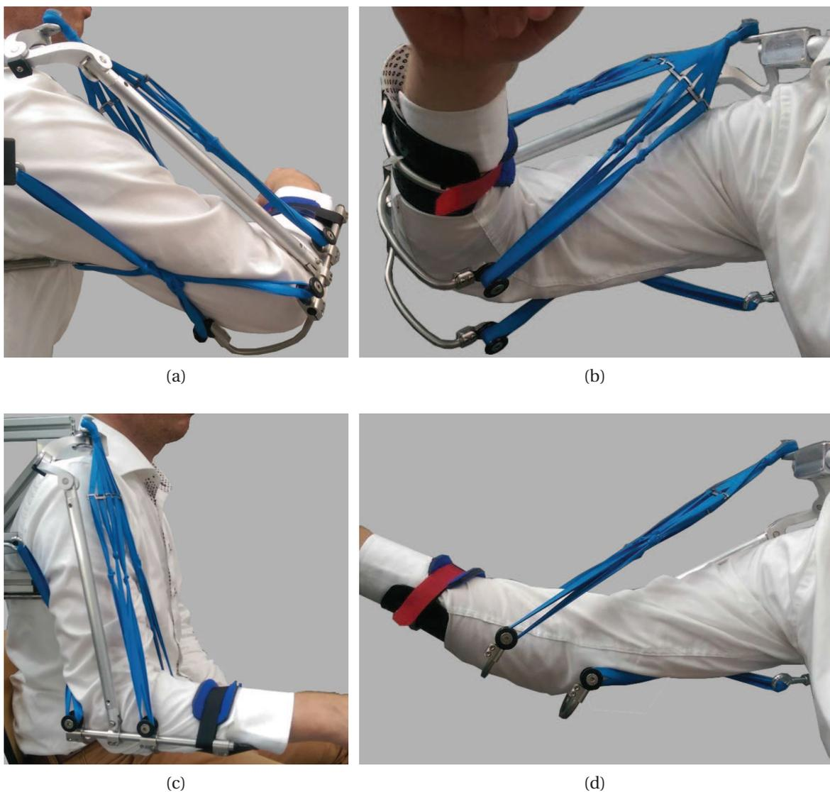
Figure 12.8: (a-d) Prototype of the 2-parallel-springs configuration, with the (a) split lower spring, and (a) split top spring.
