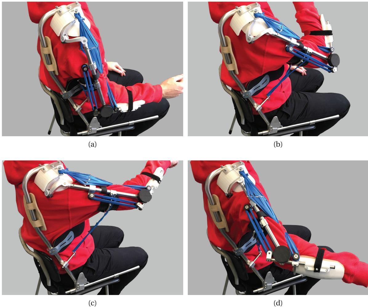
Figure 12.10: Side view of the prototype of the 3-springs configuration. In (b) and (c), the split third spring from trunk to the upper arm can be seen clearly.
