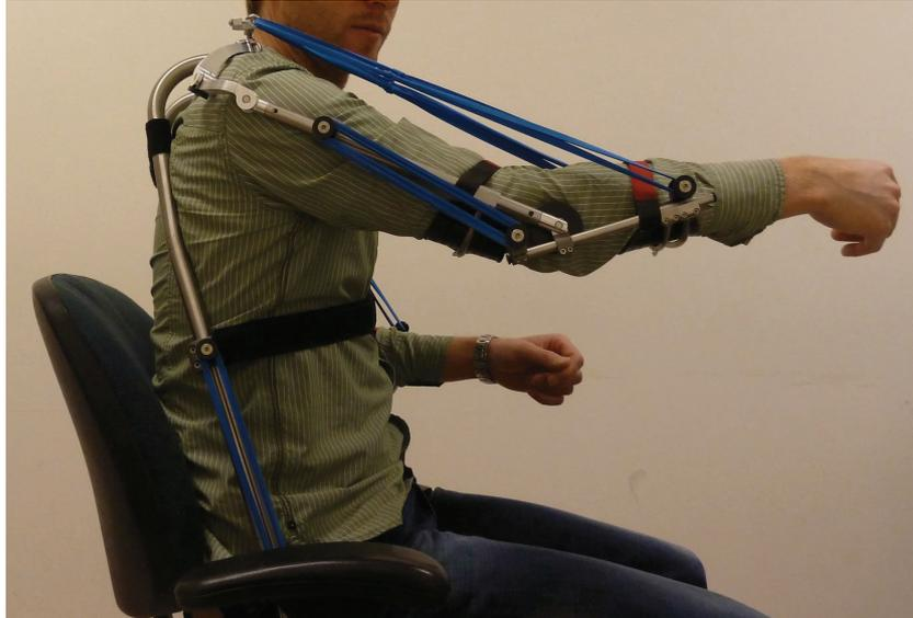
Figure 11.1: The prototype arm support worn by a healthy user.
