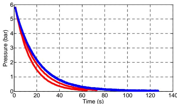
**Fig. XIV: Experimental pressure (in blue) starting at 5.83 Bar and two theoretical curves (in red), based on two different nozzle discharge factors.**
