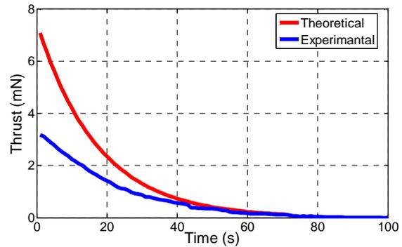
**Fig. XV Theoretical versus experimental thrust level during a blow down test with a pressure at start of 5.83 Bar.**
