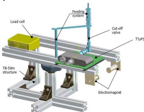
**Fig. VI: 3D model of the test setup with indication of the main features.**
