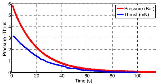
**Fig. XI: Plenum pressure history during a blow-down tests (average chamber pressure 6.5 mBar, plenum temperature 297.4 K).**
