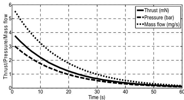
**Fig. IV Predicted thrust, pressure and mass flow rate during blow-down (with a starting pressure of 3.01 Bar).**
