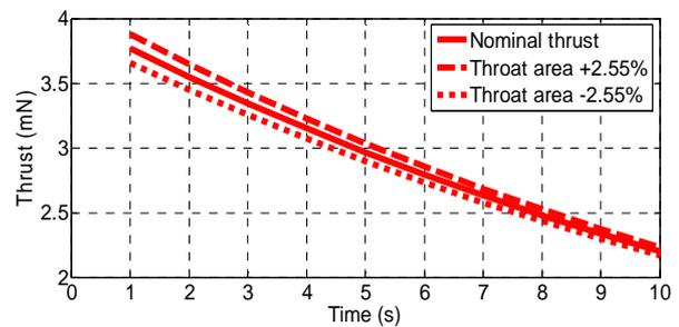
**Fig. V: Effect of uncertainty in throat area on thrust.**
