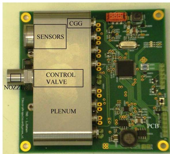
**Fig. II: Photograph of T<sup>3</sup>μPS QM**
