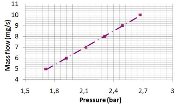
**Fig. X Mass flow versus plenum pressure from steady state testing.**
