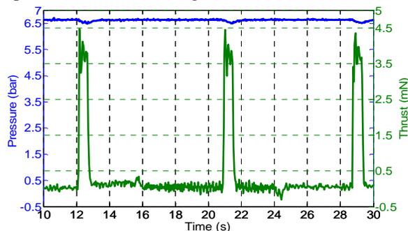
**Fig. XII: Three 500 ms impulse bits. (vacuum pressure 18 mBar, plenum temperature 297.4 K).**
