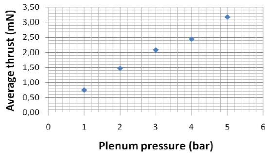
**Fig. XIII Thrust measured as function of pressure during the six blow-down tests (accuracy 15%)**
