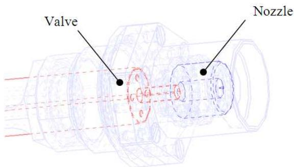
**Fig. XVII Schematic of the nozzle-valve assembly**
