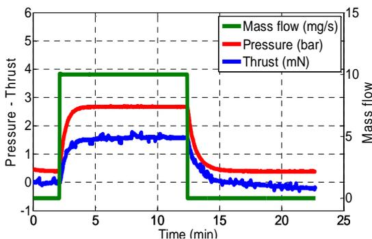
**Fig. IX: Pressure and thrust history during a steady state test at 10 mg/s; data are averaged every 10 ms (vacuum pressure 14 mBar, plenum temperature 297.4 K).**
