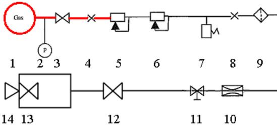
**Fig. VIII: Feeding system schematic (elements 12 to 14 are placed inside the vacuum chamber)**
