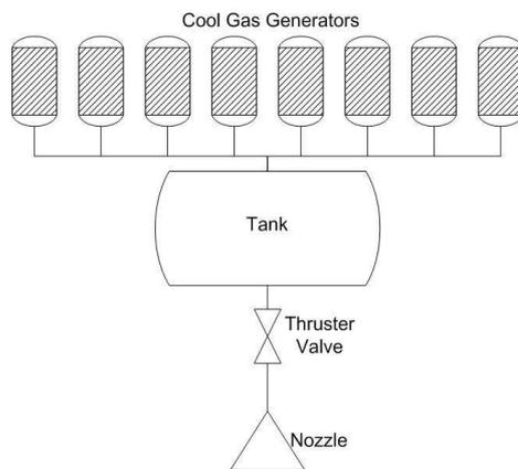
**Fig. I: Schematic of T<sup>3</sup>μPS (pressure and temperature sensor not included)**
