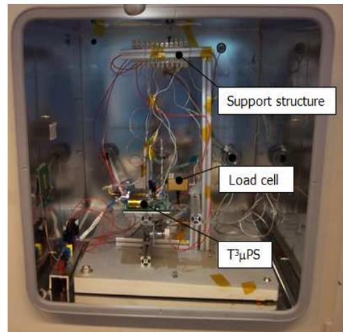
**Fig. VII: TB-50m in vacuum chamber. A support structure for electrical wires and gas feed tubing can be seen on the right and on top. Calibration over the range of interest (1-6 mN) showed an accuracy of the thrust measurement of ± 15%.**
