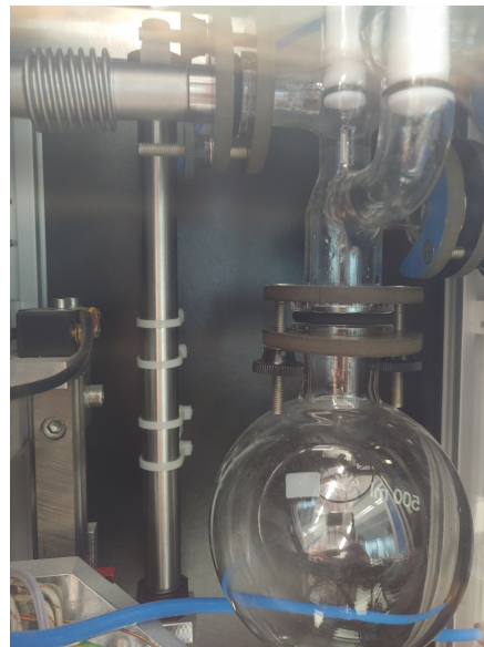
(b) View through the glass side panel of the vaporimeter, showing the tube connected to the sample tube on the left. The tubes on the top are connected to measuring devices, measuring the disturbance in the vacuum in the glass ball
