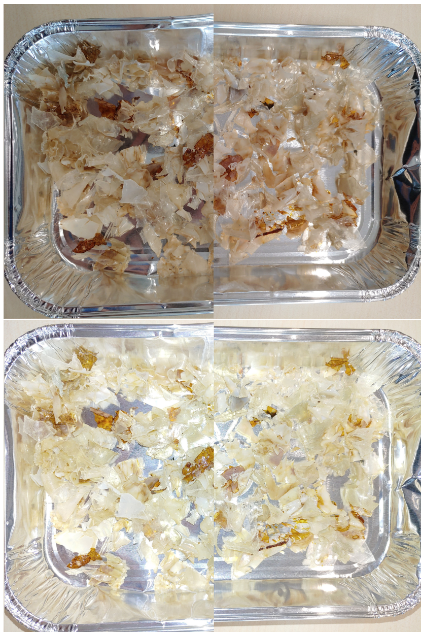
Figure 41: Combined pictures, top without flash, bottom with flash, with on the left side the roasted flakes washed with the water cooker set to 65° C and on the right side the roasted flakes with the water cooker set to 85° C
