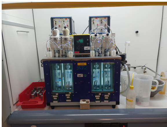
(a) Setup for four simultaneous IV measurements with four Ubbelohdes in a bath at a constant temperature of 25^{\circ}\text{C}
