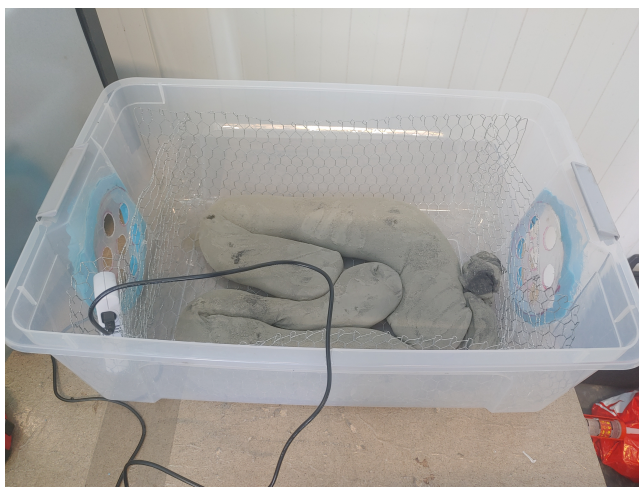
Figure 46: Portland cement in stockings inside the chicken wire cage in the dryer
