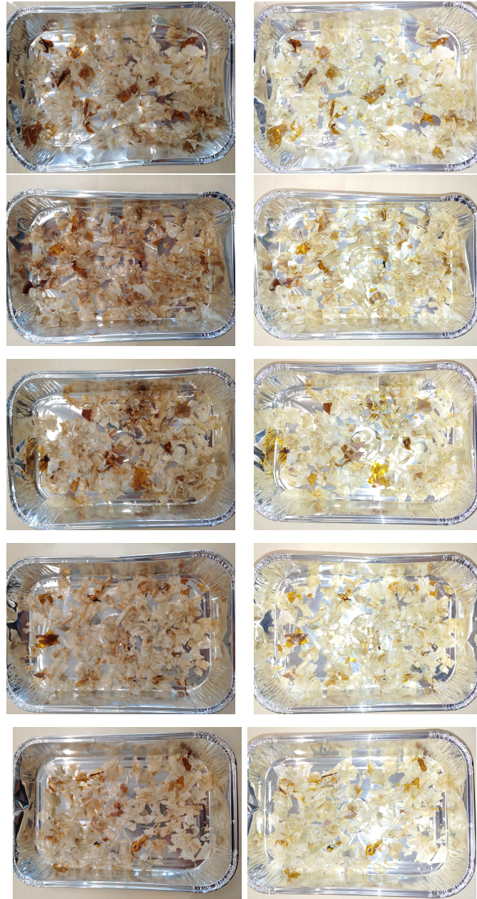
Figure 40: Pictures of the roasted flakes, pictures on the left are taken without flash and pictures on the right are taken with flash. top to bottom the temperature setting on the water cooker was 65° C, 70° C, 75° C, 80° C and 85° C
