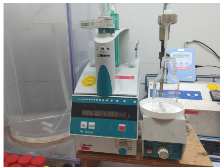
(b) DCA (left) is dispensed by the computerized solvent dispenser (middle) into the flask with specimen (right)
