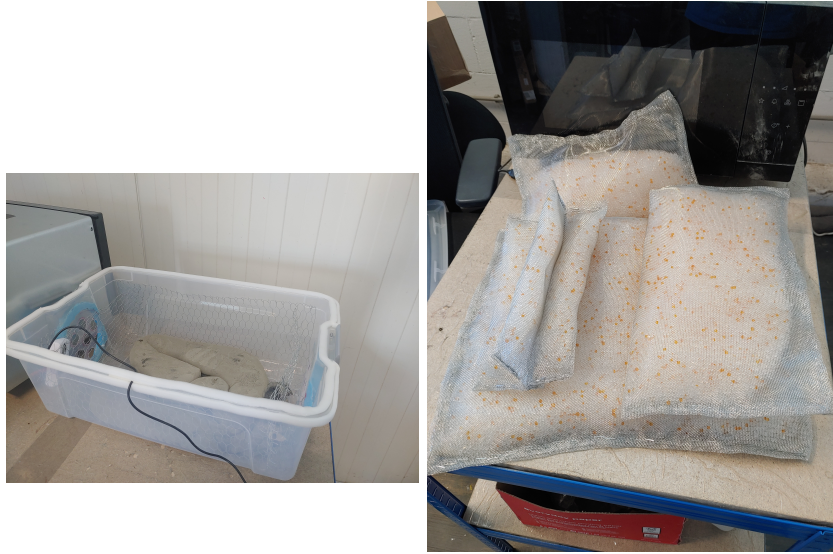
Figure 19: Building the dryer and the desiccant. In the first figure a different desiccant, Portland cement, can be seen, which was an earlier iteration of the design. See appendix III for more information
