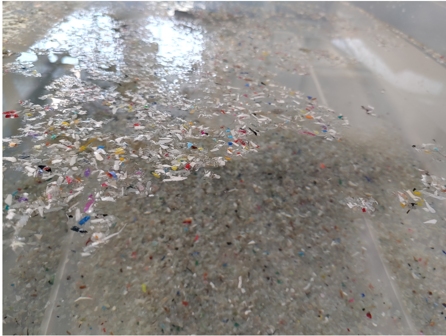
Figure 39: Sink-float analysis of the fines in a large container, showing most fines sink
