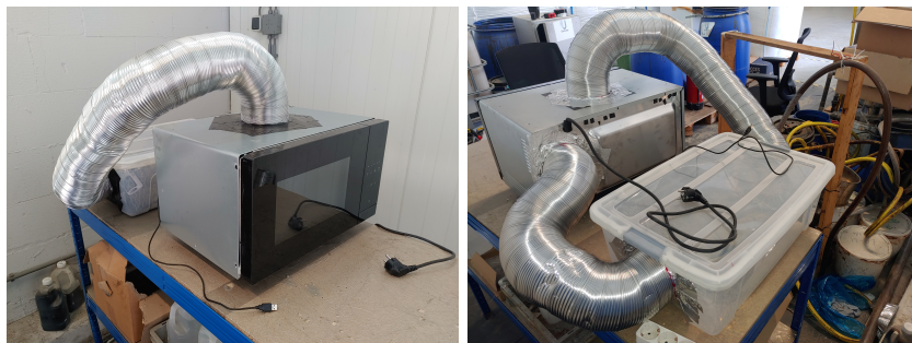
Figure 20: Finished research setup from two angles, showing both the microwave plug and the thermo-hygrometer data cable
