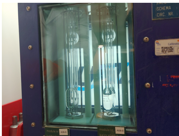
(b) View through the glass panel, showing two Ubbelohdes in more detail
