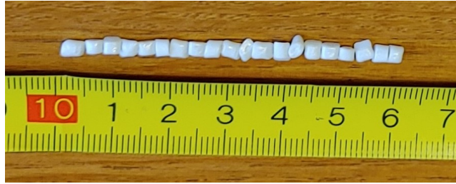
Figure 28: Size measurement of 20 pellets show an average radius of 4mm
