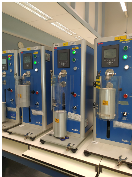
(a) Three vaporimeters shown from the front. The left and right vaporimeter have the heating element over the specimen, whereas the middle vaporimeter has the heating element positioned down
