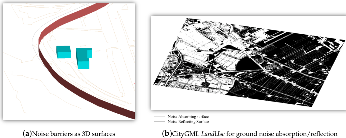
Figure 11. Noise barriers and ground types in the generated 3D city model.
