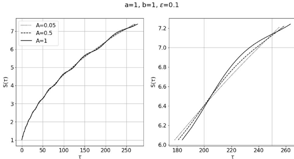
**Fig. 6.** Position of the moving boundary in case of a periodic temperature at the fixed endpoint for different values of  $A$ . The left figure is the position from initial time and the right one is a zoom-in at the  $\tau$ -interval  $[200, 250]$ .
