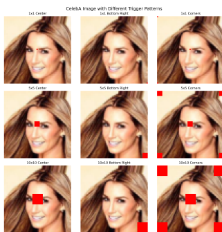
Figure 4: Image showing the 9 different triggers of sizes 1x1, 5x5, and 10x10 positioned in the center, the bottom right corner, and all four corners as well as the center of the image.
