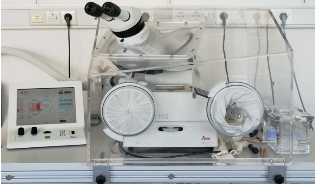
SF 3.1: An anti-contamination glove box surrounds the cryo-ultramicrotome. The chamber is used to reduce contamination in and around the microtome while vitreous cryo-sectioning. With a steady influx of dry nitrogen gas and dry sodium hydroxide pellets the humidity within the chamber can be reduced to below 1% RH.
