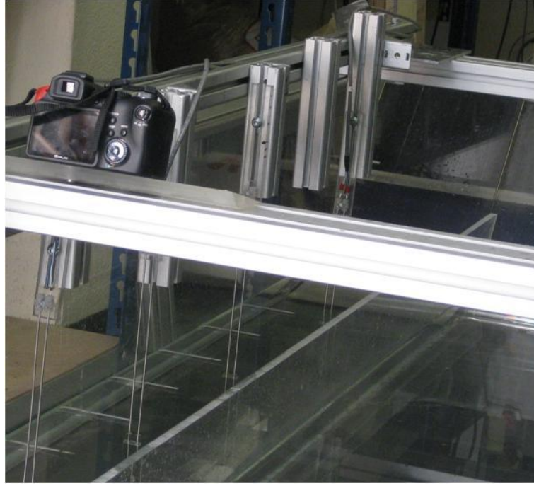
Figure 3.8 Wave channel: the camera and the resistance wave probes
