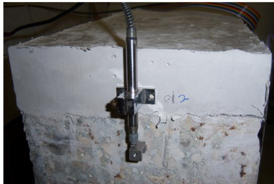
Figure 4.2 LVDT measuring the interface delamination.
