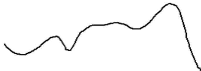
a. Measured profile of the grit-blasted surface
