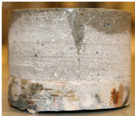
Figure 4.4 FRPM specimen for RCM tests.
