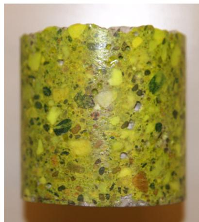
Figure 5.2 Specimen for capillary absorption test.
