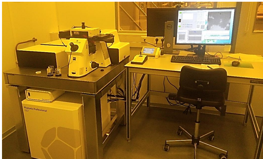
Figure 2: Nanoscribe Photonic Professional (GT) laser lithography system at the Micro- and Nano-engineering department (MNE) of the Mechanical, Materials and Maritime Faculty (3ME) of the TU Delft.
