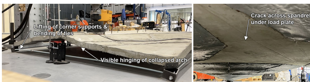
Fig. 14 Visible support rotation and tie bending accompanied by a visible collapse of the arch (left) and cracking of the spandrel underneath the load plate (right) observed during the MN1M test
