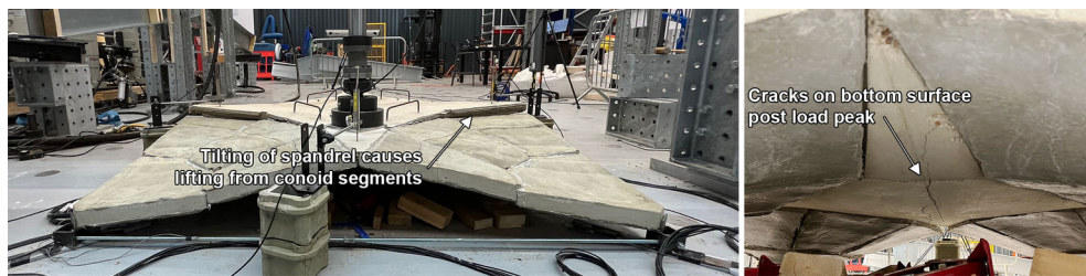
Fig. 15 Lifting of spandrel from conoid segments due to tilting (left) and cracking of the spandrel underneath (right) observed during the MN2M test
