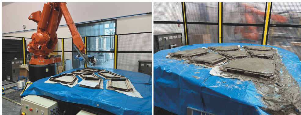
Fig. 10 Spraying of a quarter of the conoid segments for the 1st shell prior to (left) and after (right) the GFRC is deposited
