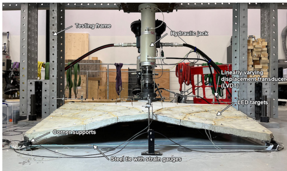
Fig. 12 Assembled MN1 shell prior to testing
