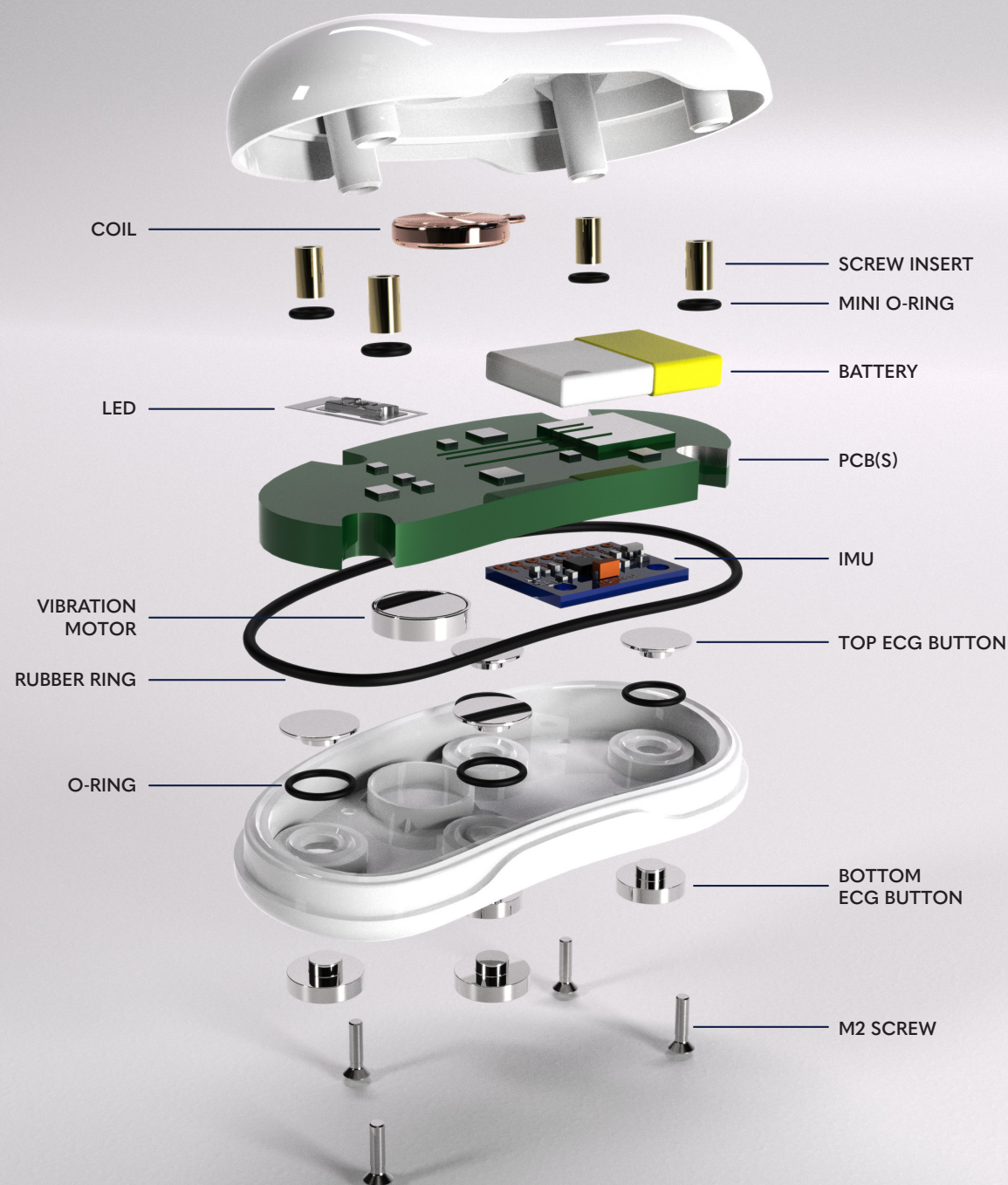
FIGURE 57: EXPLODED VIEW OF THE DEVICE
