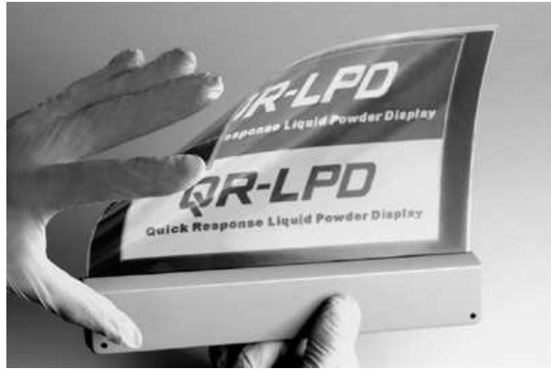
Figure 4.1: A QR-LPD display developed by the Bridgestone Corporation.
