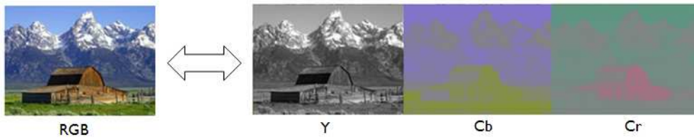
Figure 5.5: Example of RGB and YCbCr Format
