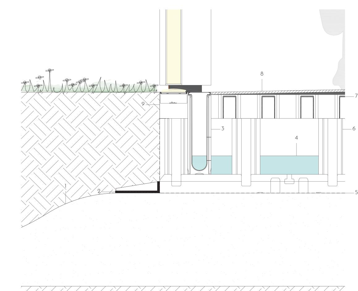
road elements with integrated lighting and gutter | 1:5
