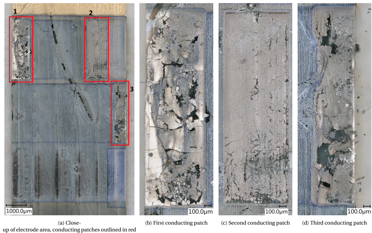
Figure 6.11: (a) section of laser sintering experiments, (b)-(d) close-ups of conducting patches
