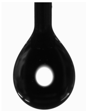
Figure 5.5: Pendant drop test with PDMS:OA 1:4 ink, image captured at maximum volume
