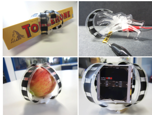
Figure 1.3: Gripper that closes upon actuator, wrapped around various objects, taken from [7]
