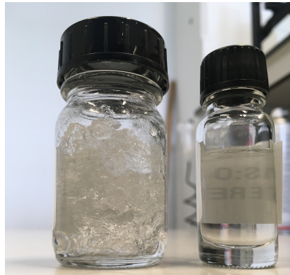
Figure 5.6: PDMS:OA 1:4 solutions stored in two different types of container, prepared on the 29th of September (right bottle) and on the 10th of October (left bottle). The left mixture has solidified, whereas the ink on the right is still fluid.
