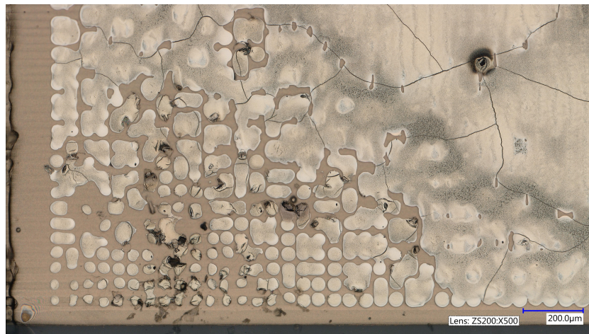
Figure 6.6: Close-up of an electrode printed five hours after surface treatment
