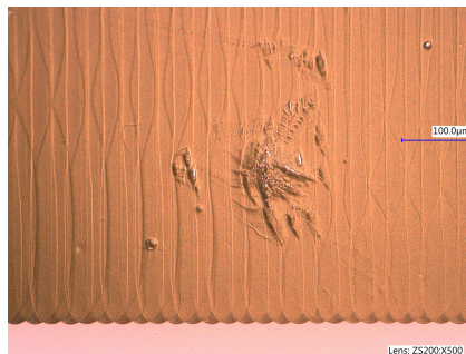
Figure 3.2: Mitsubishi NBSIJ-MU01 printed over a dust particle on the substrate
