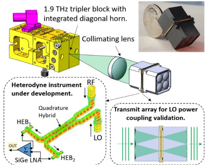
**Fig. 1.** Schematic showing LO coupling to a  $2 \times 2$  pixel heterodyne array, integrated in a silicon micromachined package. By slightly modifying the wafer-stack into a transmit array configuration, allows for validating the efficiency of LO coupling and RF antenna performance.
