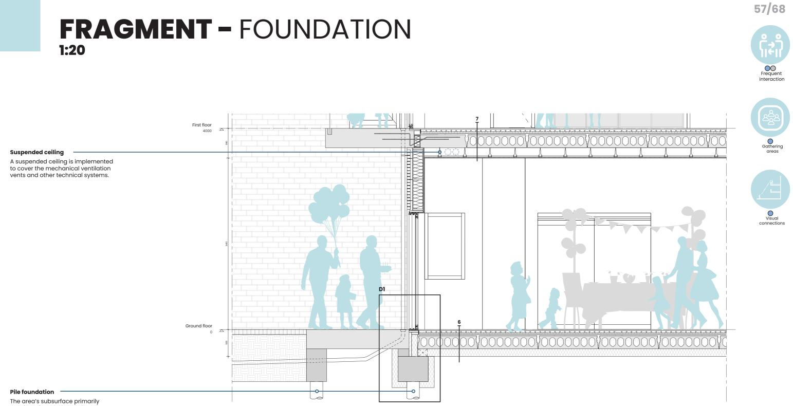
The area's subsurface primarily consists of weak clay and peat layers, which lack the necessary bearing capacity. Therefore, a pile foundation is needed.
