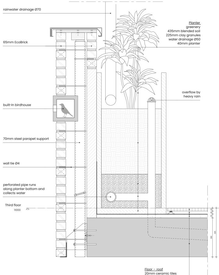
20mm tile carriers waterproof membrane 25mm concrete screed 260 solid concrete slab
