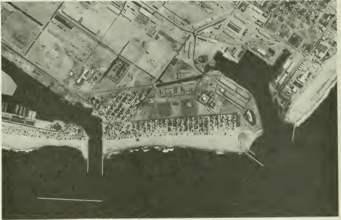
(Photo was taken just after 2.3 million cubic meters of sand had been dredged from the trap, Sept. 1965.)
