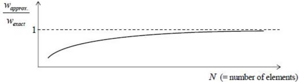
Figure 4.6 The accuracy increases when the mesh refines (Blauwendraad, 2006)
