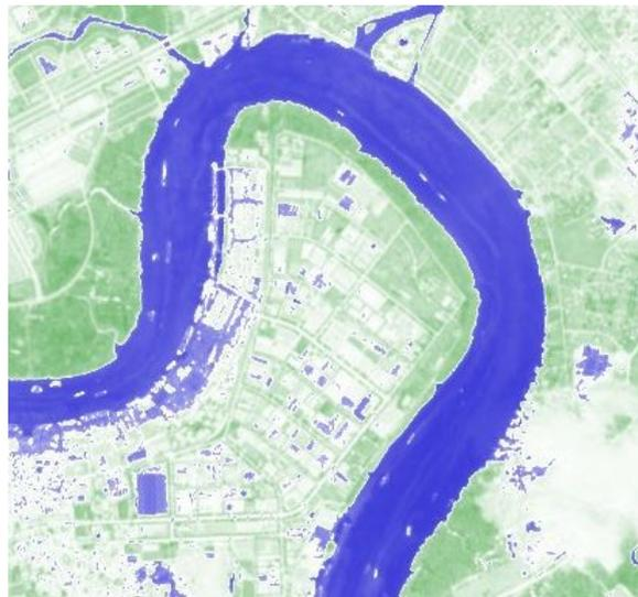
Figure B.3: Satellite image of the Saigon river, Vietnam of the normalized difference water index (NDWI)
