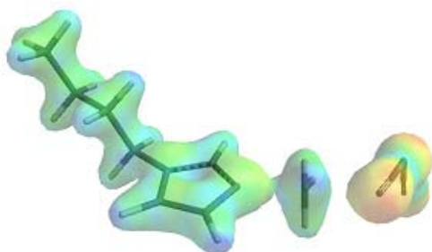
Figure 7.10: Transition state geometry (via s_N2 ) of the thermal breakdown of [bmim][N(CN) 2 ] into butylimidazole and methylated dicyanamide (surface = electron density of 0.08 e/au 3 ; property = electrostatic potential). The electron density is high at the red positions (large negative values of the potential) and low at the blue positions (large positive values of the potential).
