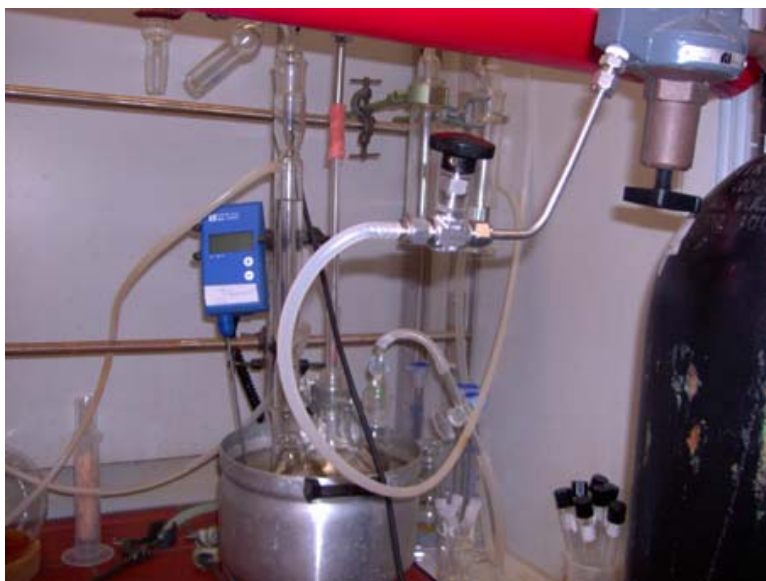
Figure 4.4: Experimental set-up for the preparation of [bmim][Cl] from 1-methylimidazole and 1-chlorobutane
