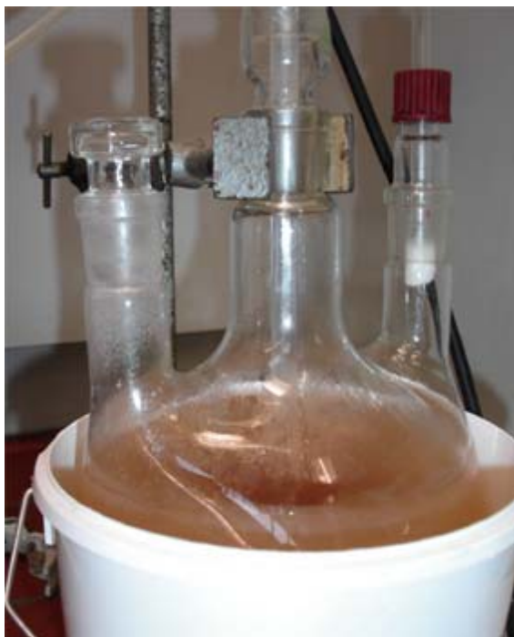
Figure 4.5: Experimental set-up for the preparation of [bmim][BF 4 ] from [bmim][Cl] and sodium tetrafluoroborate
