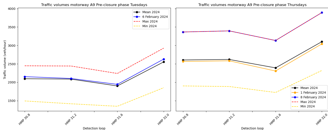
Figure 23: Pre-closure (19:00 - 20:00) traffic volumes A9 motorway
