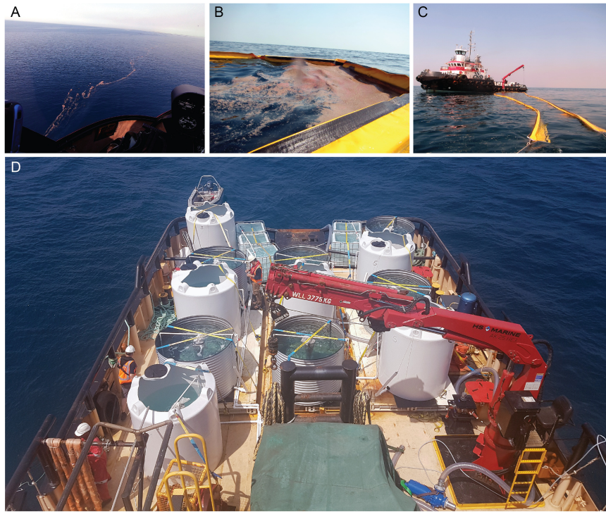
FIGURE 1 | Testing the feasibility of operationalizing the spotting, containing, collecting, and culturing of coral-spawn slicks at industrial-scales. (A) View of a spawn slicks in the open ocean from a helicopter. (B) Containing coral-spawn slick in an oil boom for (C) collection onto the tugboat. (D) Overview of the back deck of the tugboat with the 4,500 L steel ( n = 6 ) and plastic ( n = 6 ) tanks.
