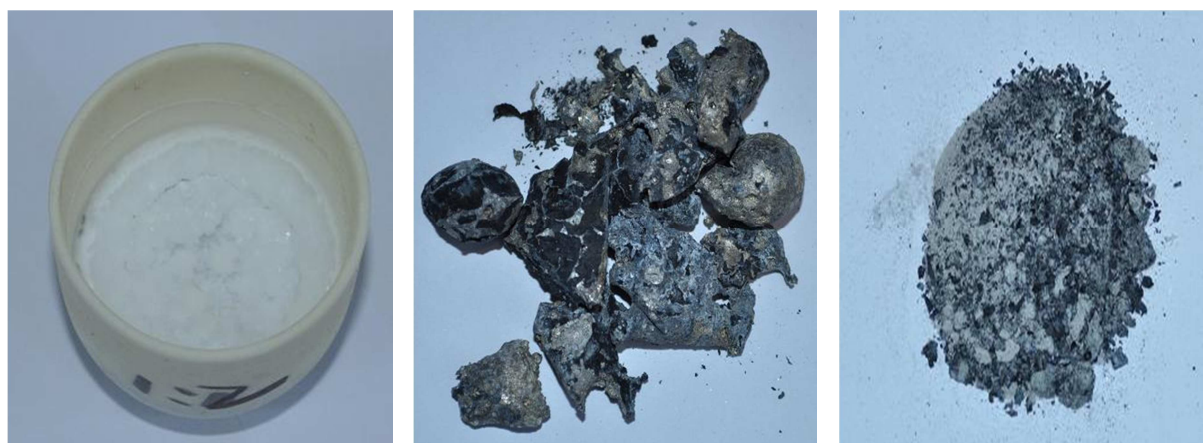
Figure 4.24: Experiment C2: salts-to-alloy ratio 2:1 with \text{MgF}_2 in crucible after melting (left), obtained alloy (middle) and non metallic contaminants (right).
