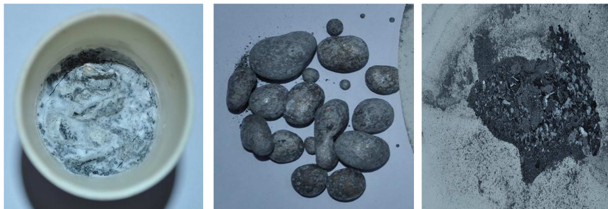
Figure 4.28: Experiment C3: salts-to-alloy ratio of 1:1 and 10% \text{Na}_3\text{AlF}_6 in crucible after melting (left), obtained alloy (middle) and slag (right).
