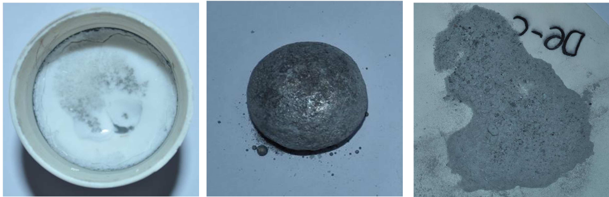
Figure 4.37: Experiment E1, de-coated scrap with a salts-to-alloy ratio of 2:1, in crucible after melting (left), obtained alloy (middle) and non metallic inclusions (right).
