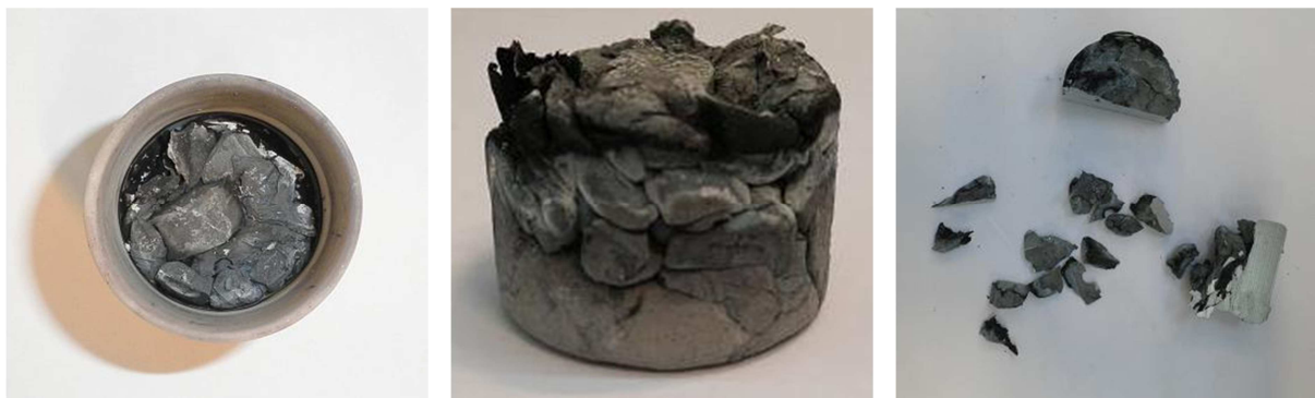
Figure 4.38: Experiment E2, not de-coated scrap without a salt flux, in crucible after melting (left), obtained alloy (middle) and after sawing (right).
