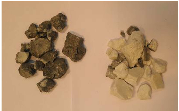
Figure 4.18: Salt slags from experiments A3 for not de-coated alloy (left) and A6 for de-coated alloy (right).
