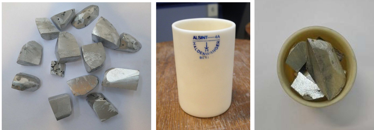
Figure 3.7: Sawed and polished alloy (left), 4 cm diameter Alsint crucible (middle) and alloys in the crucible (right).
