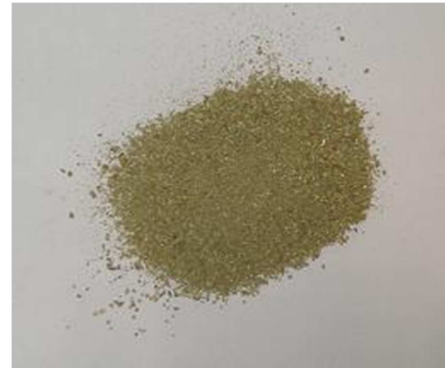
Figure 4.2: Powder from sieving the de-coated scrap.
