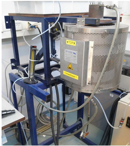
Figure 3.3: Tube furnace with an argon gas lance on top.
