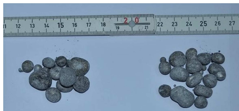
Figure 4.30: The aluminium alloy particles from experiments C3 (right) and C4 (left) with a scale.
