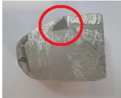
Figure 4.33: Small piece of titanium in the Al-alloy.
