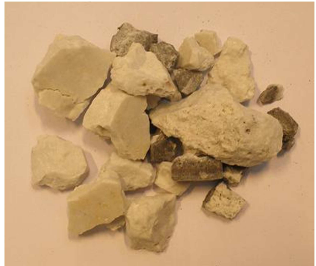
Figure 4.17: Salt slag after experiment A6.
