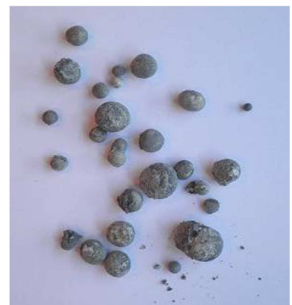
Figure 4.11: The small alloy particles from within the salt flux.
