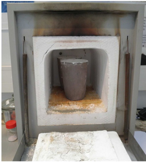
Figure 3.2: Pre-melting and de-coating furnace for small samples.
