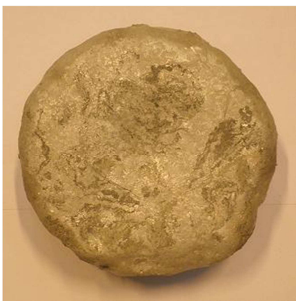
Figure 4.9: Top surface of the recovered metal alloy.
