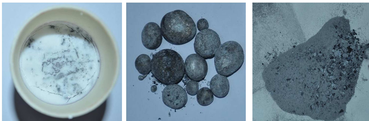
Figure 4.4: Experiment A1, not de-coated scrap with a salts-to-alloy ratio of 2:1, in crucible after melting (left), obtained alloy (middle) and non metallic contaminants
