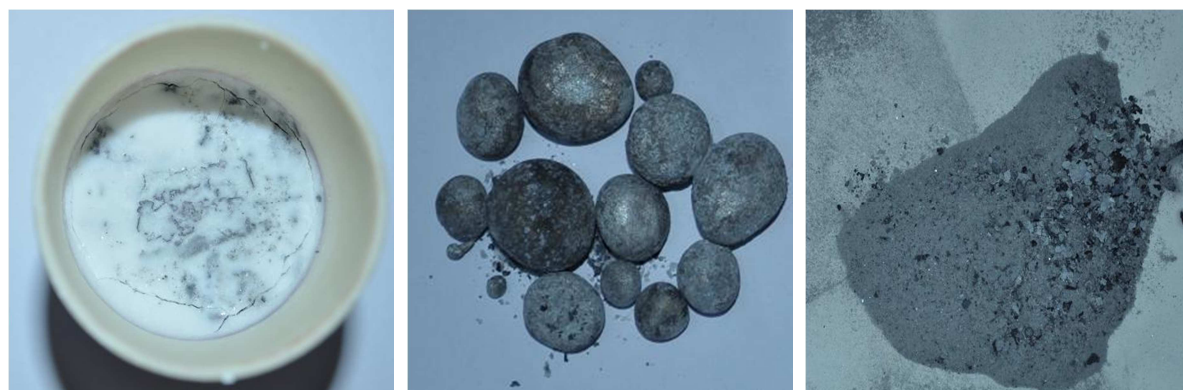
Figure 4.20: Experiment B2: salts-to-alloy ratio 2:1 with 10% \text{Na}_3\text{AlF}_6 in crucible after melting (left), obtained alloy (middle) and non metallic inclusions (right).
