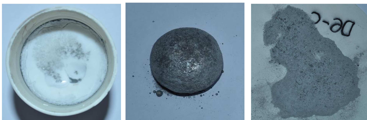
Figure 4.5: Experiment A2, de-coated scrap with a salts-to-alloy ratio of 2:1, in crucible after melting (left), obtained alloy (middle) and non metallic contaminants (right).
