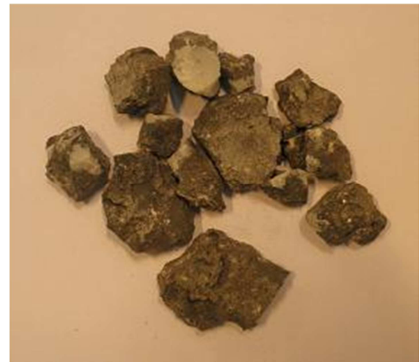
Figure 4.13: Salt slag after melting of not de-coated scrap.
