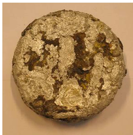
Figure 4.10: Bottom side of the recovered metal alloy.
