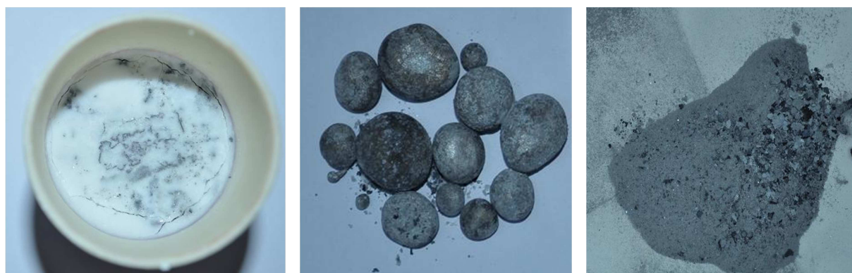
Figure 4.29: Experiment C4: salts-to-alloy ratio 2:1 and 10% \text{Na}_3\text{AlF}_6 in crucible after melting (left), obtained alloy (middle) and slag (right).
