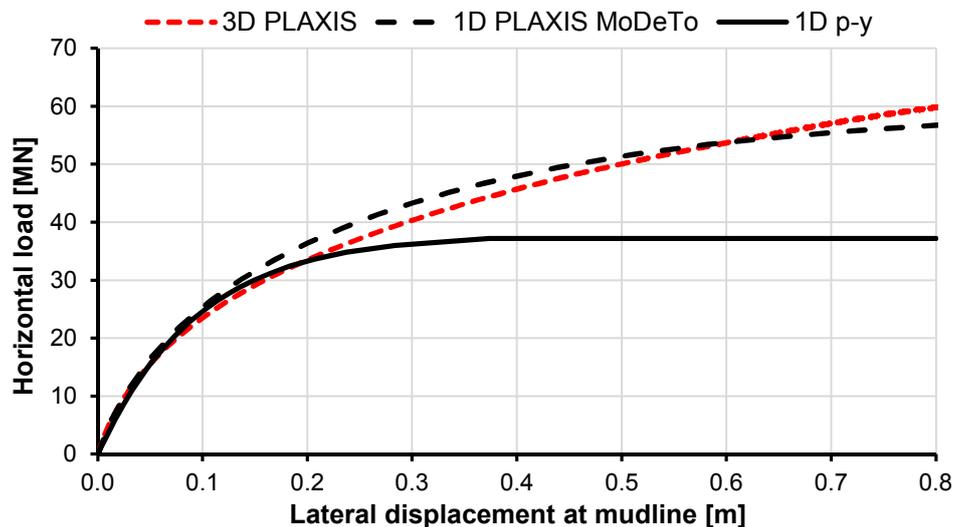
Fig. 3. Horizontal load versus lateral displacement at mudline for the design model
